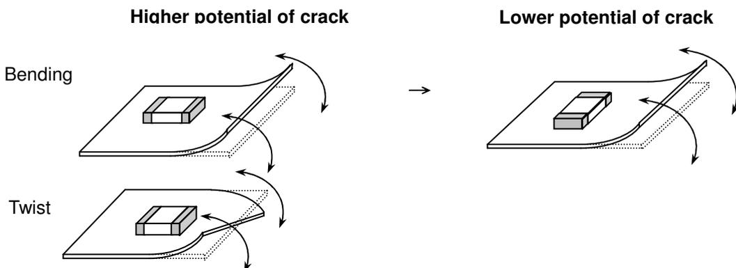
5.2 There is a potential of crack if board is warped due to excessive load by check pin
