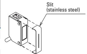
Horizontal slits and round slits have an orientation. Make sure that the TOP marking comes on top of the sensor (LED side).
