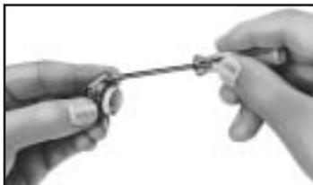
The translucent filter in the lens holder can not be removed because this filter is sealed to make the unit waterproof and oiltight.
