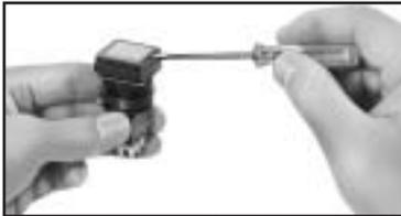
2. Remove the marking plate by pushing the lens from the rear to disengage the latches between the lens and the lens holder, using the screwdriver as shown below.
