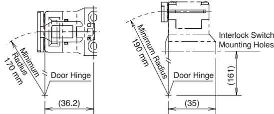
When the door hinge is on the extension line of the actuator mounting surface:
