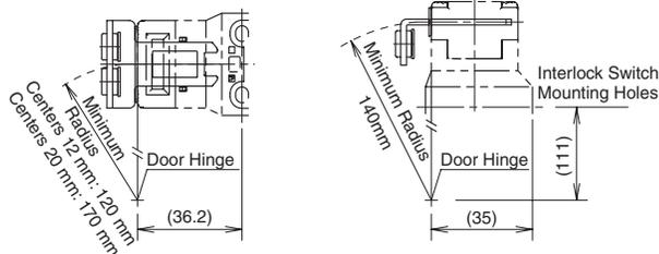
When the door hinge is on the extension line of the actuator mounting surface:
