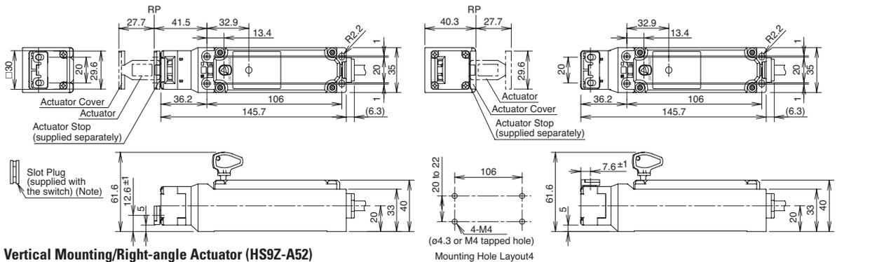
**Vertical Mounting/Right-angle Actuator (HS9Z-A52)**
