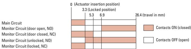
The operation characteristics shown in the chart above are of the HS9Z-A51. For other actuator types, add 1.3 mm.
