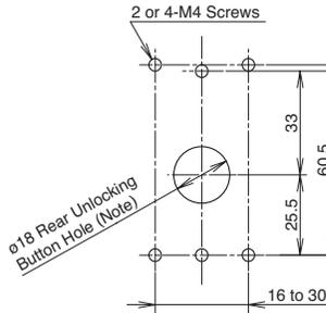
Note: With the mounting hole dimension, the rear unlocking button rod does not touch the hole even when the interlock switch moves sideways.
