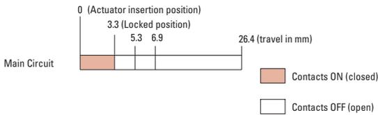
The operation characteristics shown in the chart above are of the HS9Z-A51. For other actuator types, add 1.3 mm.
