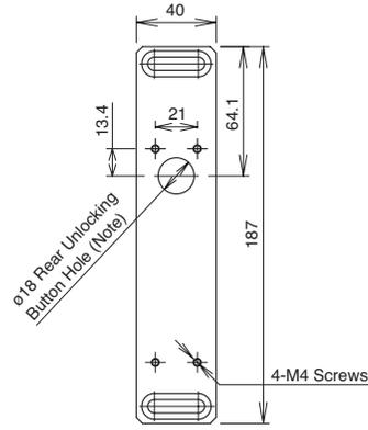
When installing the HS5E-□44□-G (rear unlocking button type), provide a rear unlocking button hole on the HS9Z-SP51.
