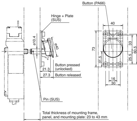
Rear Unlocking Button Kit Mounting Hole Layout
