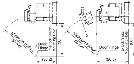
When using the HS9Z-A55 Angle Adjustable (vertical/horizontal) Actuator
