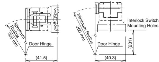
HS9Z-A52 Actuator (w/rubber bushings)
