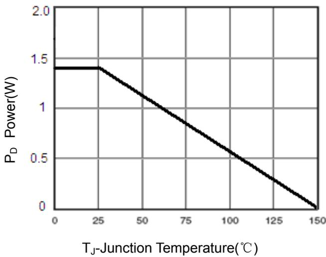
Figure 3 Power Dissipation
