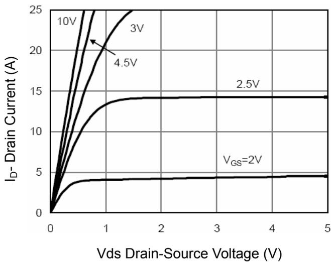
Figure 5 Output Characteristics
