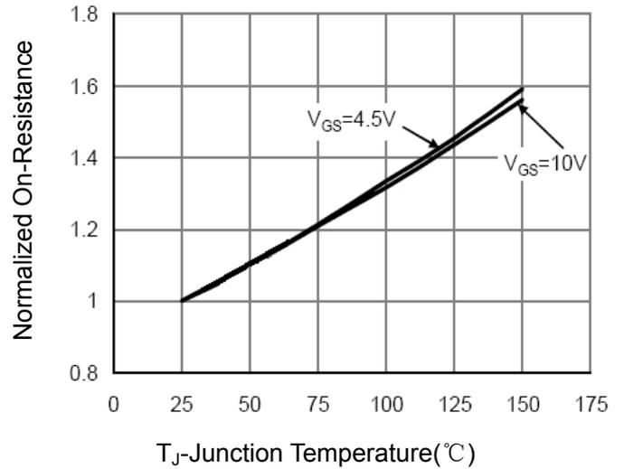
Figure 8 Drain-Source On-Resistance
