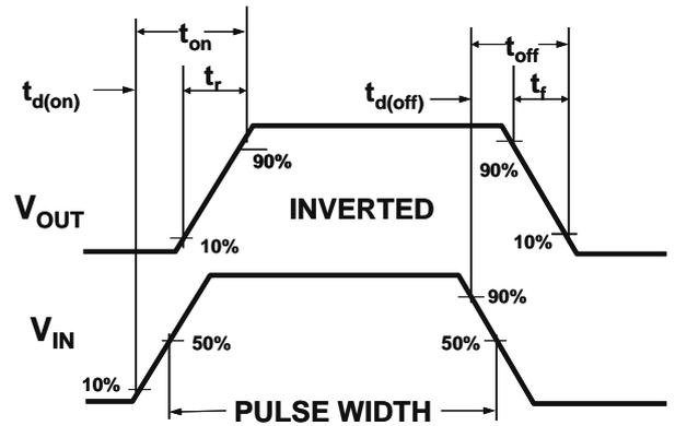
Figure 2: Switching Waveforms
