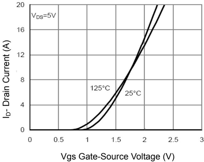
Figure 7 Transfer Characteristics
