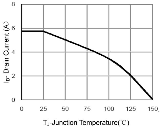
Figure 4 Drain Current
