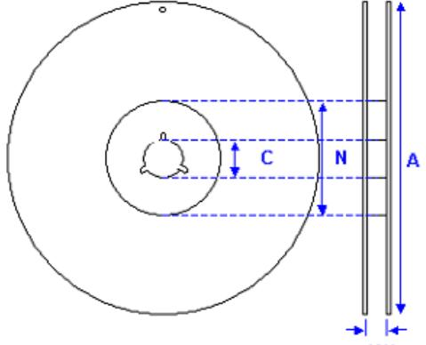
The diagram illustrates a reel with two concentric circles. Dimension 'A' is the outer diameter of the reel. Dimension 'C' is the distance from the center to the inner edge. Dimension 'N' is the inner diameter of the reel. Dimension 'W1' is the width of the reel.
