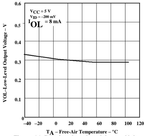
**Figure 14. Receiver Low-Level Output Voltage vs Free-Air Temperature**
