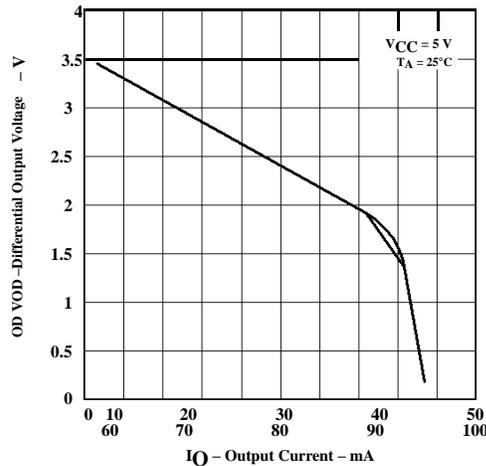
**Figure 10. Driver Differential Output Voltage vs Output Current**
