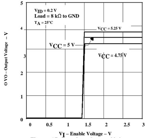
**Figure 15. Receiver Output Voltage vs Enable Voltage**
