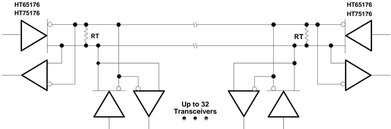
The line should be terminated at both ends in its characteristic impedance ( $R_T = Z_0$ ). Stub lengths off the main line should be kept as short as possible.
