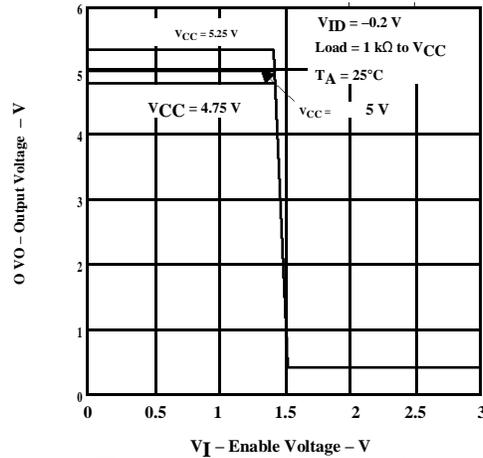
**Figure 16. Receiver Output Voltage vs Enable Voltage**
