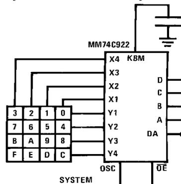
Outputs are enabled when valid entry is made and go into 3-STATE when key is released.
