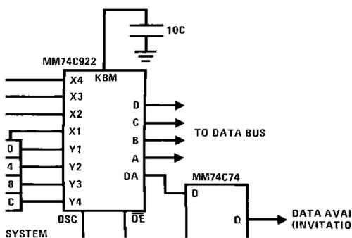
The keyboard may be synchronously scanned by omitting the capacitor at osc. and driving osc. directly if the system clock rate is lower than 10 kHz
