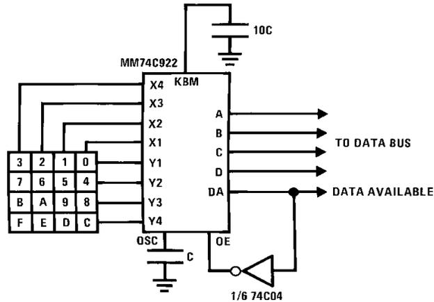
Outputs are in 3-STATE until key is pressed, then data is placed on bus. When key is released, outputs return to 3-STATE.
