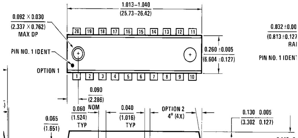
20-Lead Plastic Dual-In-Line Package (PDIP), JEDEC MS-001, 0.300 Wide
