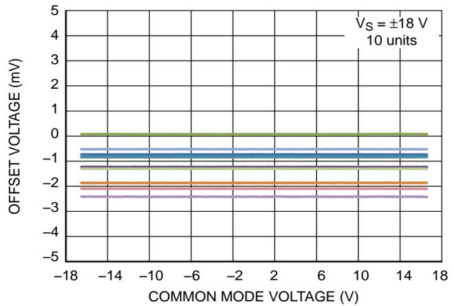
**Figure 5. Input Offset Voltage vs. Common Mode Voltage**
