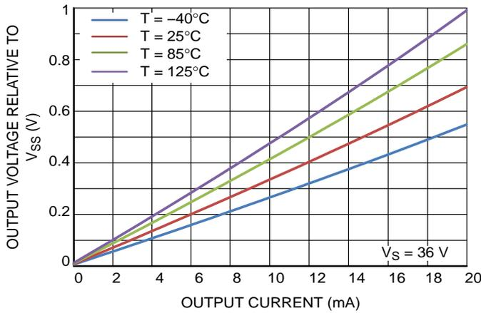
Figure 16. Low Level Output vs. Output Current
