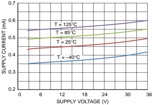
**Figure 2. Quiescent Current Per Channel vs. Supply Voltage**
