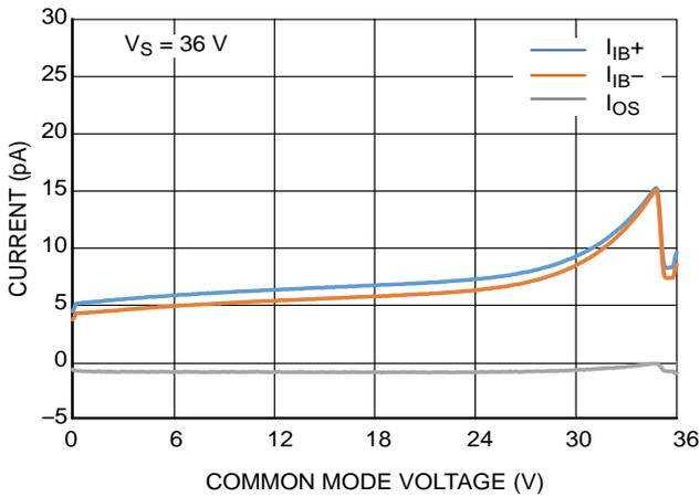
**Figure 22. Input Bias Current vs. Common Mode Voltage**
