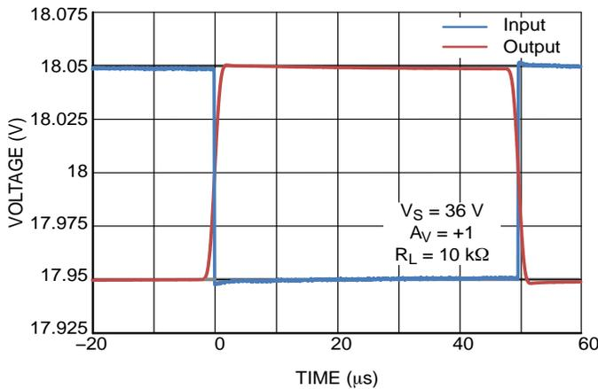
Figure 18. Inverting Small Signal Transient Response
