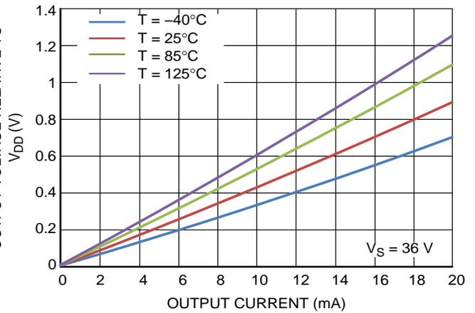
Figure 15. High Level Output vs. Output Current
