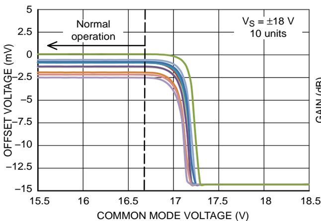
**Figure 6. Input Offset Voltage vs. Common Mode Voltage**
