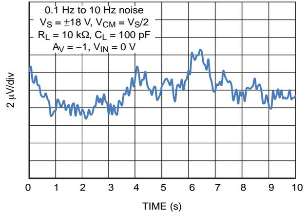
**Figure 23. 0.1 Hz to 10 Hz Noise**
