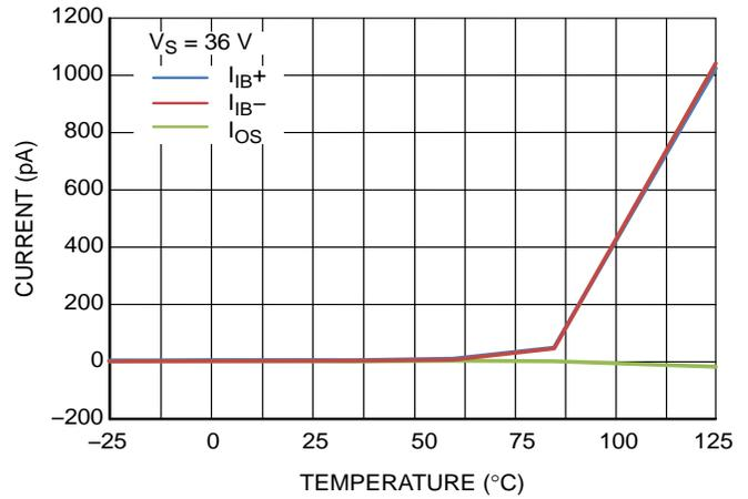
**Figure 21. Input Bias and Offset Current vs. Temperature**
