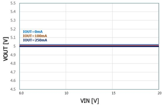
VIN=6.0V to 20V, VOUT=5.0V @ IOUT=0A/100mA/250mA
