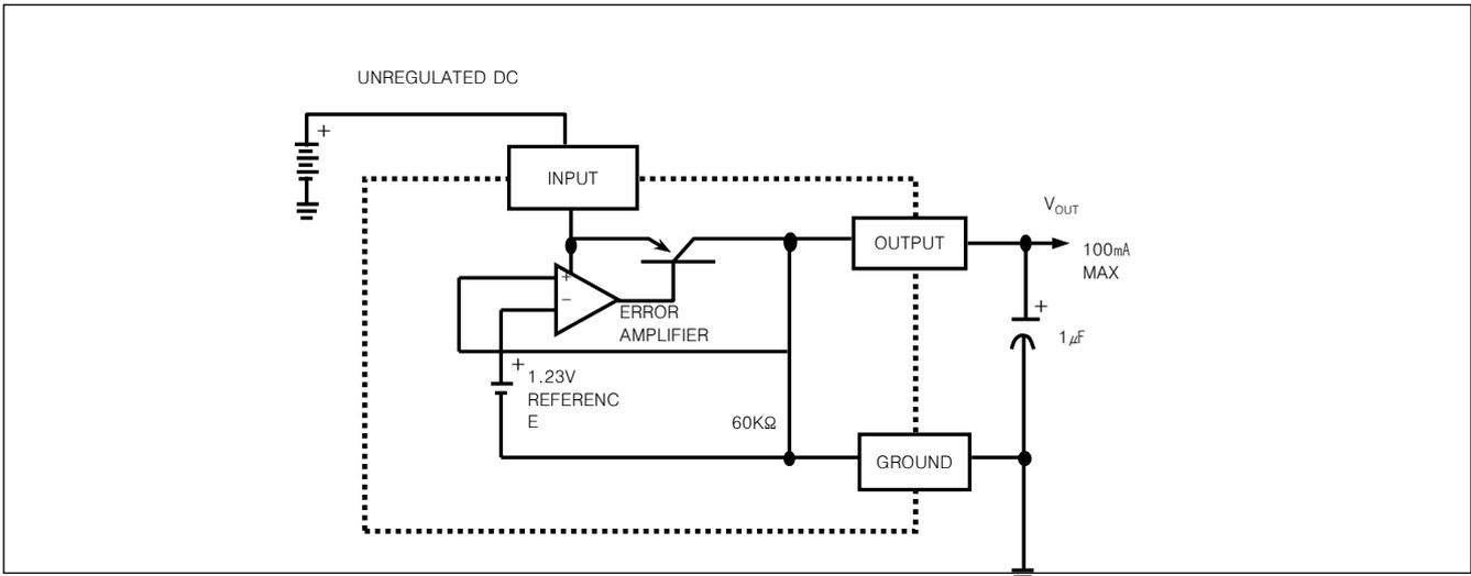
**BLOCK DIAGRAM AND TYPICAL APPLICATIONS (LM2951)**
