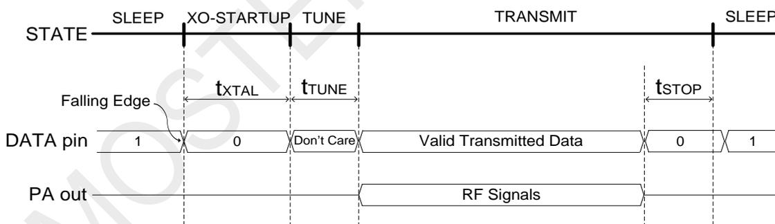
Figure 17. Transmission Enabled by DATA Pin Falling Edge
