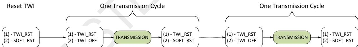
Figure 19. CMT2110/17A Operation Flow with TWI
