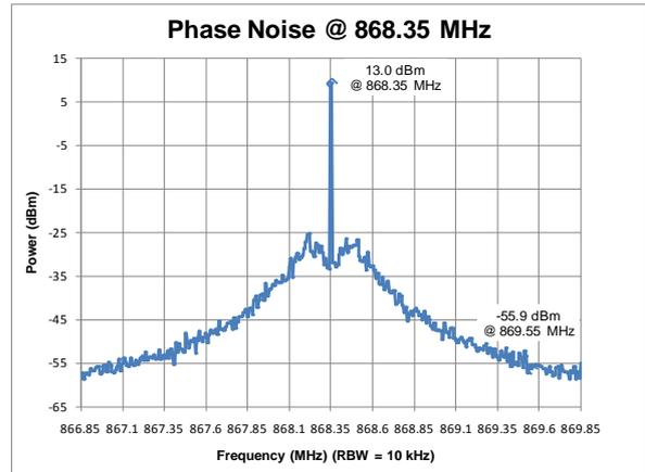
**Figure 4. Phase Noise,  $F_{RF} = 868.35$  MHz,
