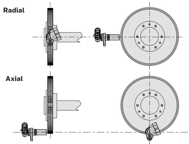
Figure 4. SNG-QPLA-000 Mounting Dimensions (For reference only: mm/[in].)
