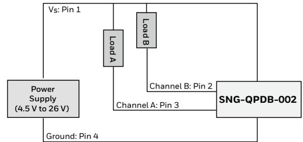
Note: The load resistor values should be such that the output current does not exceed the maximum load current of 40 mA.
