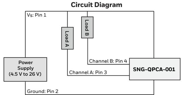
Note: The load resistor values should be such that the output current does not exceed the maximum load current of 40 mA.
