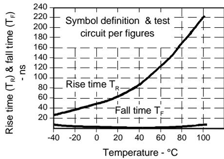
Fig. 4 Delay Time vs Temperature gra\_062.ds4
