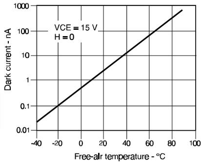
Fig. 4 Collector Current vs Ambient Temperature
