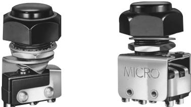
An elastomer seal is bonded between actuating plunger and button collar. An O-ring seals the button assembly to the panel front.
