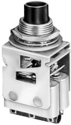
These pushbuttons are equipped with HM hermetically sealed switch units, which have metal-to-metal fusion around the cover, actuator base, and mounting holes. Terminals are sealed glass-to-metal.
