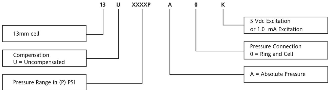
For example: **Part #13U 3000PA0K** = 13 mm Cell, Uncompensated, 3000 psi, Absolute, Ring pressure connection with 5 Vdc excitation.
