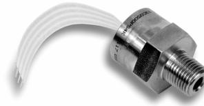
Honeywell's 13 mm Series stainless steel pressure sensors are designed for high pressure applications that involve measurement of hostile media in harsh environments. This series uses Honeywell's proven piezoresistive semiconductor sensor chip in an oil-isolated housing with or without an integral ceramic for temperature compensation and calibration. This design has proven to be highly reliable, stable and accurate.
