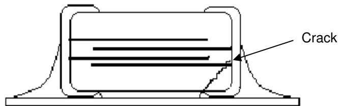
**6. Handling of Loose Chip Capacitor**
