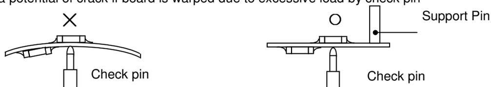
5.3 Mechanical stress due to warping and torsion.
