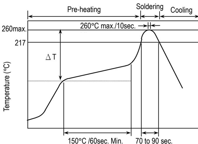
※ The cycles of soldering : Twice (max.)
