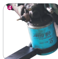
• Oil filter removal & assembly
