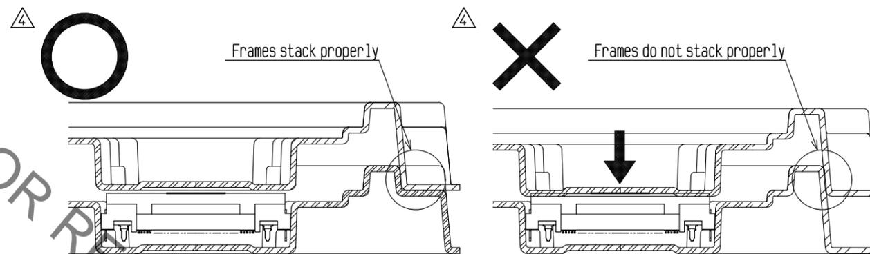
If the tray is stacked correctly, tray's frame prevents from upper tray applying force to the connector on bottom tray.
