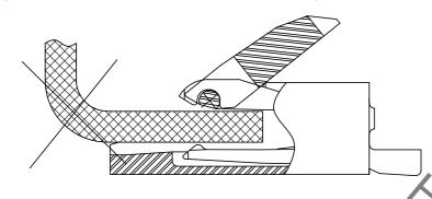
5. When inserting an FPC, do not use the method shown in the figure on the left below where the corner of the FPC is inserted first and then slid sideways. the FPC's corner can deform the terminal's contacts. Always insert the FPC parallel to the board as shown in the figure on the right below.
