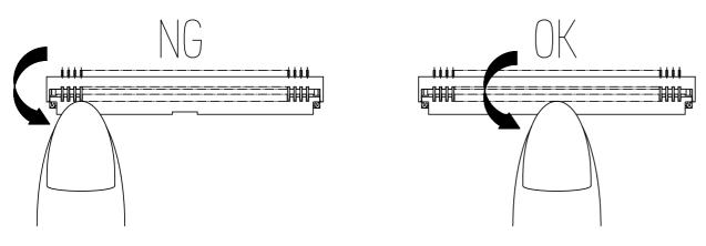
♦ Confirming the state of the lock Once it is locked, make sure that the actuator is parallel to the board. However, if the actuator approaches O degrees, make sure that it is not.
