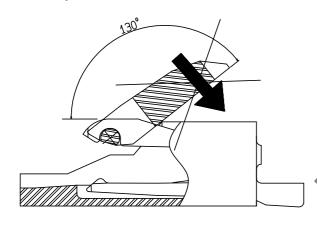
4. When operating the actuator, avoid operating it at its end. Make sure to operate it at its middle section.
