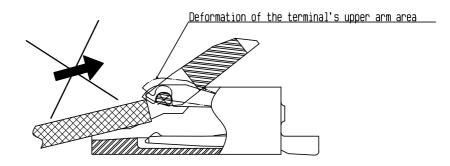
3. Do not insert the FPC at an angle. Do not insert the FPC from above at an angle as shown in the figure. This may cause the FPC to bend or the terminal to deform. Additionally, the FPC may not insert all the way and result in discontinuation.
