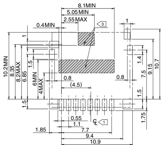
Note 1 indicates the center line of the microSD card slot.
