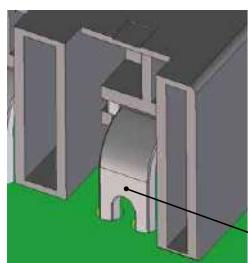
Since the lead mounting part has some exposed parts, please insure sufficient clearance when mounting other parts near this connector.
