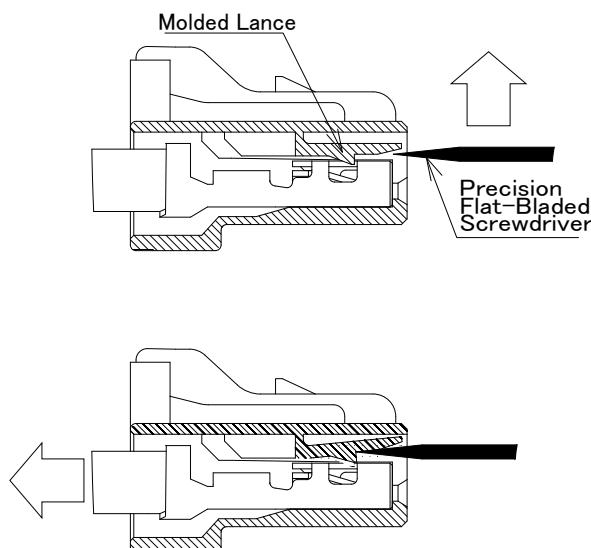
1. After unmating the parts, position the flat-bladed screwdriver to raise the lance as shown in the illustration.
