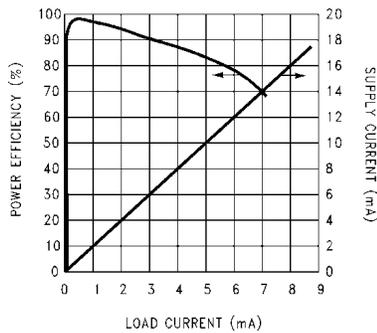
**Supply Current & Power Efficiency vs Load Current (V<sup>+</sup> = 5V)**
