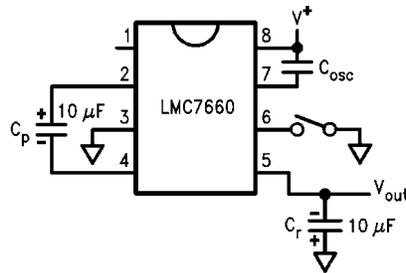
FIGURE 3. Reduce Supply Current by Lowering Oscillator Frequency
