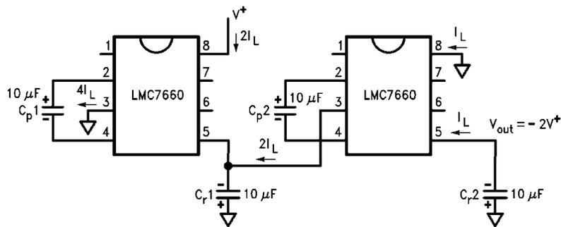
FIGURE 6. Higher Voltage by Cascade
