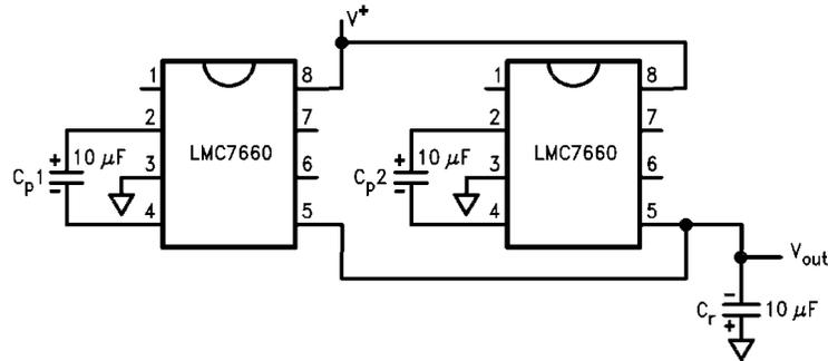
FIGURE 5. Lowering Output Resistance by Paralleling Devices
