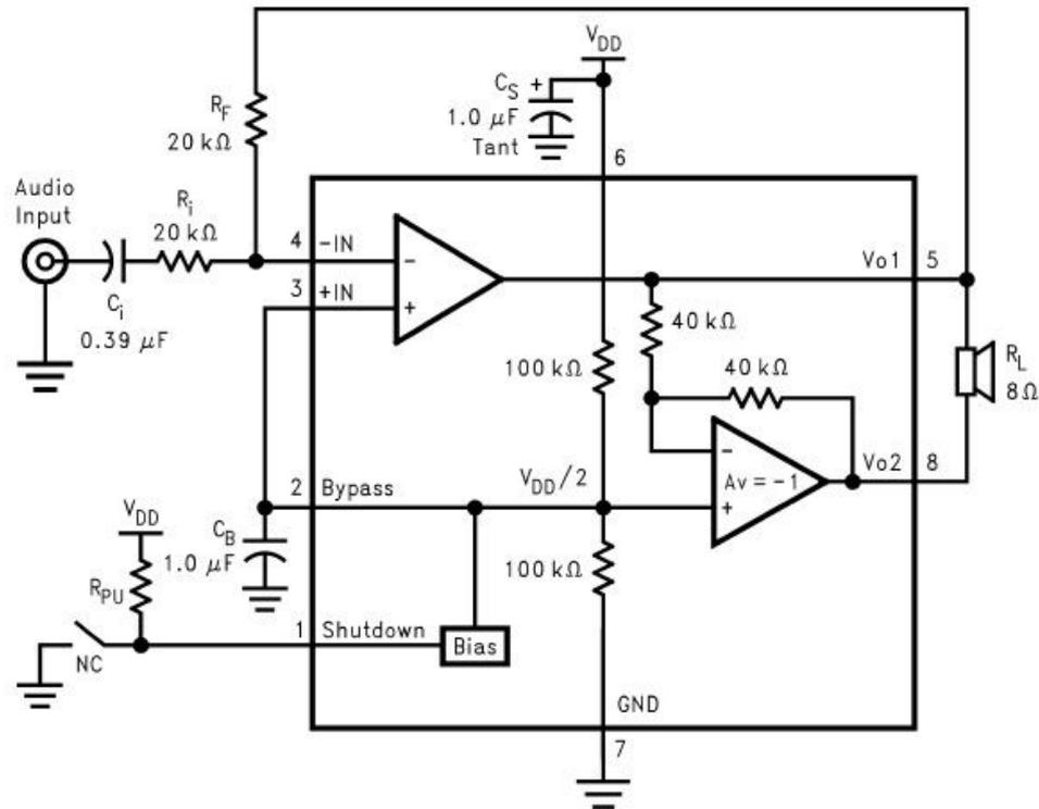
Figure 3. Typical Audio Amplifier Application Circuit
