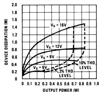
Device Dissipation vs Output Power — 16 $\Omega$  Load
