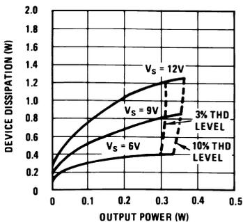
Device Dissipation vs Output Power — 8 $\Omega$  Load
