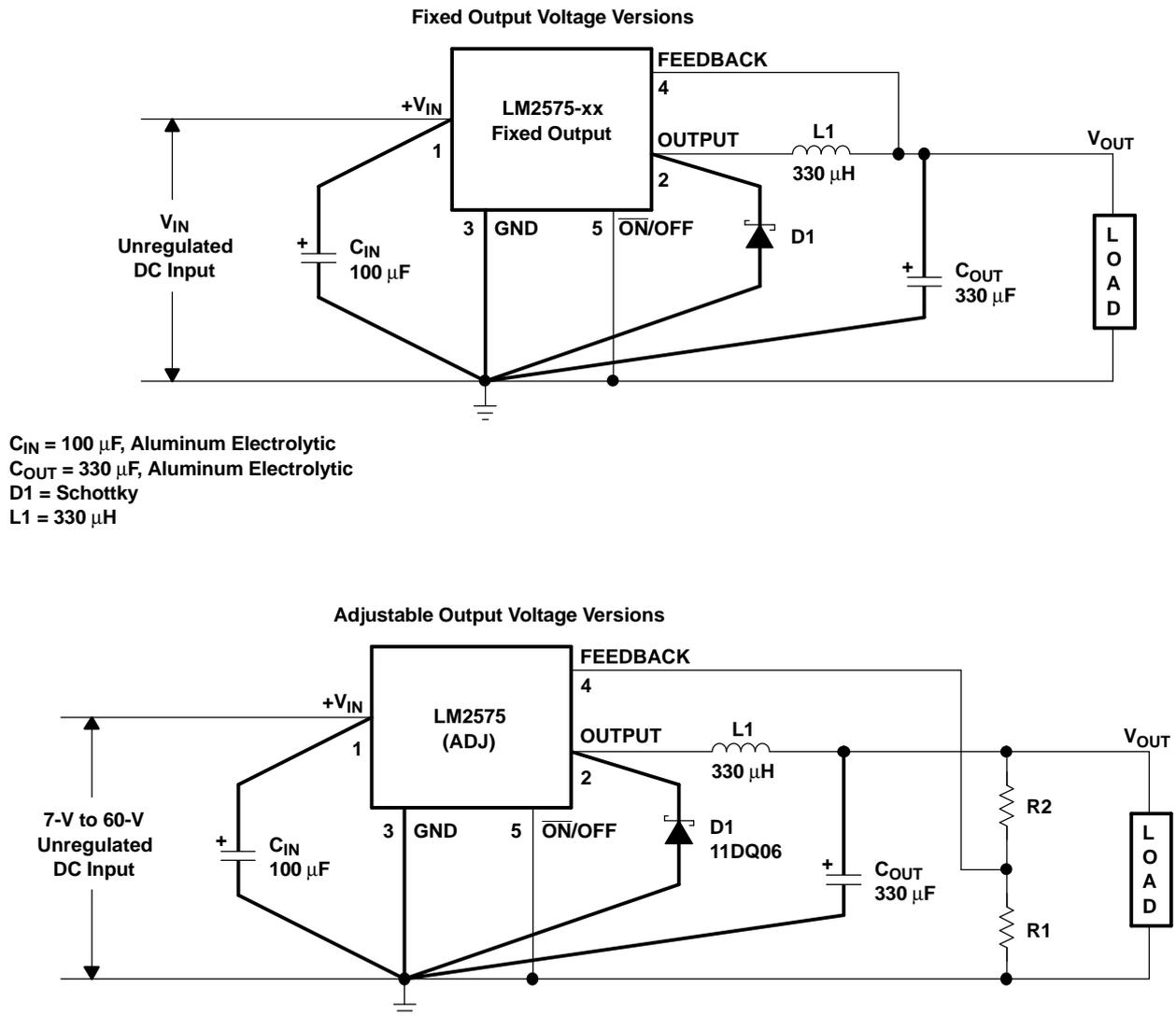
$C_{IN} = 100 \mu\text{F}$ , Aluminum Electrolytic
