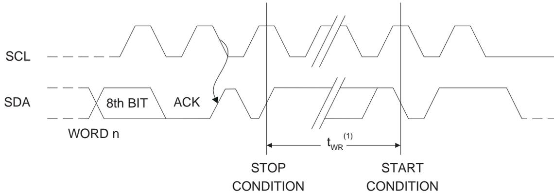
Note: 1. The write cycle time  $t_{WR}^{(1)}$  is the time from a valid stop condition of a write sequence to the end of the internal clear/write cycle.
