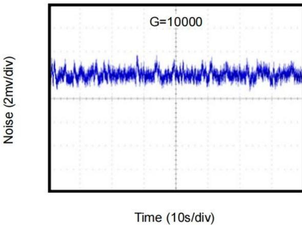
0.1Hz to 10Hz Noise at +2.5V
