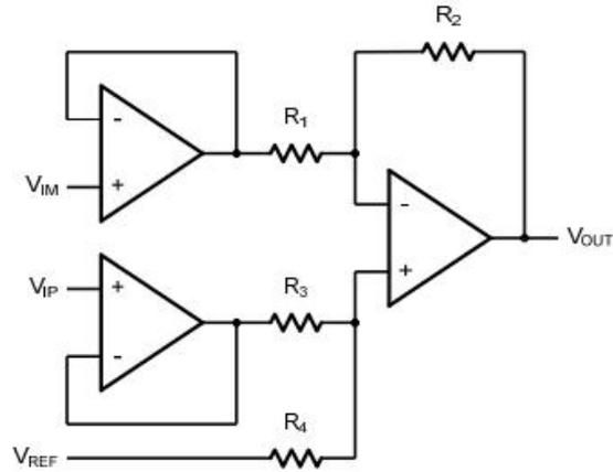
Figure 6. Instrument Amplifier
