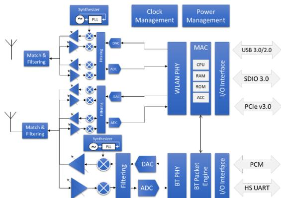
The SPB228 is highly integrated and its complete and proven system functionality means quicker design cycles at lowest risk and simplified, cost efficient manufacturing. The 28nm design reduces power consumption and supports advanced signal processing that enhances link robustness and supports transmit beamforming for increased capacity and range.
