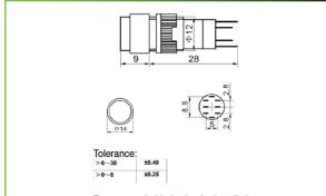
Recommended hole size for installation: Ø12mm
