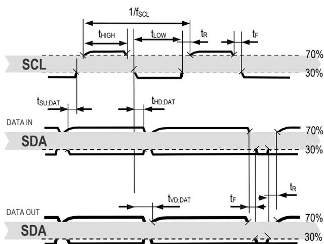
**Figure 5** Timing diagram for digital input/output pads. SDA directions are seen from the sensor. Bold SDA lines are controlled by the sensor, plain SDA lines are controlled by the micro-controller. Note that SDA valid read time is triggered by falling edge of preceding toggle.
