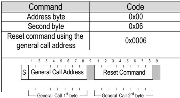
**Table 12** Reset through the general call address (Clear blocks are controlled by the microcontroller, grey blocks by the sensor).
