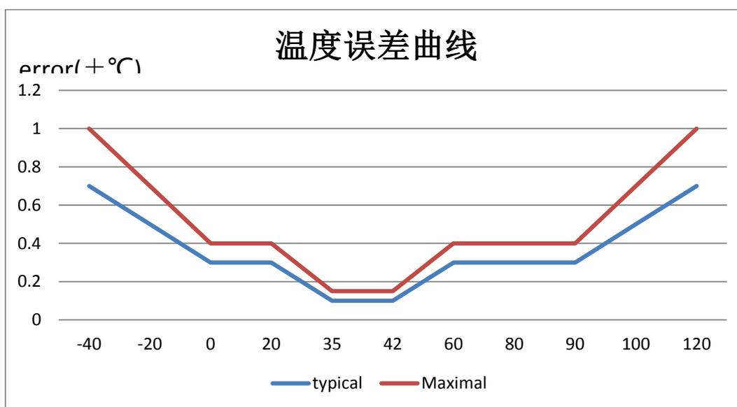
Figure 2 Temperature accuracy of the GXTS03 sensor.
