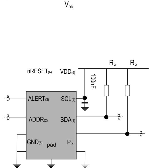
**Figure 4** Typical application circuit. Please note that the positioning of the pins does not reflect the position on the real sensor. This is shown in Table 5.
