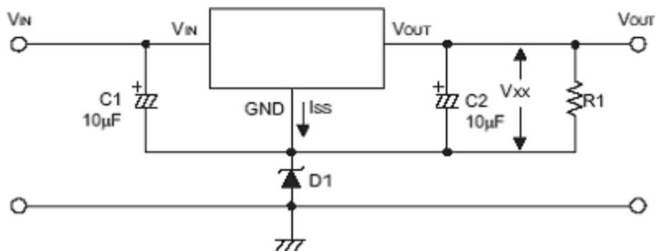
$$V_{OUT} = V_{xx} + VD1$$
