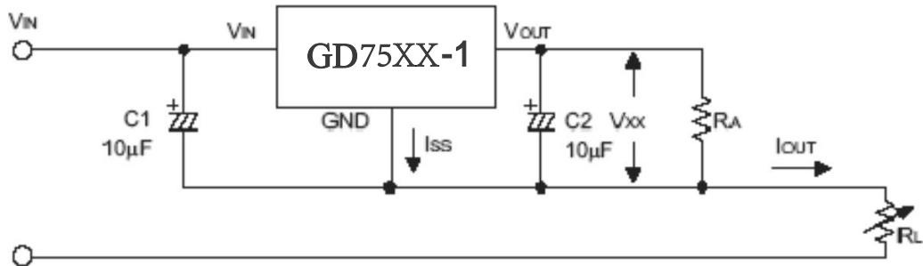
$$I_{OUT} = V_{xx}/R_L + I_{SS}$$
