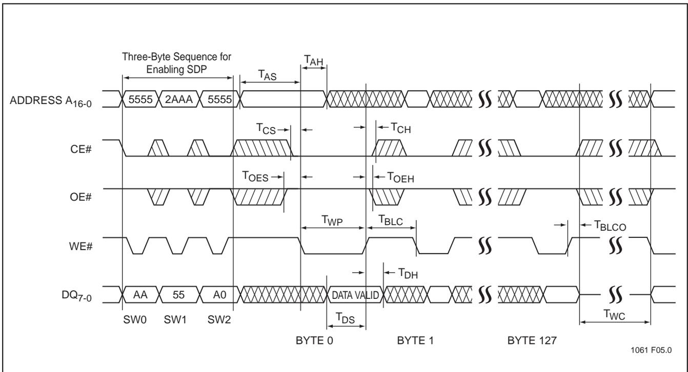
**FIGURE 6: WE# Controlled Page-Write Cycle Timing Diagram**
