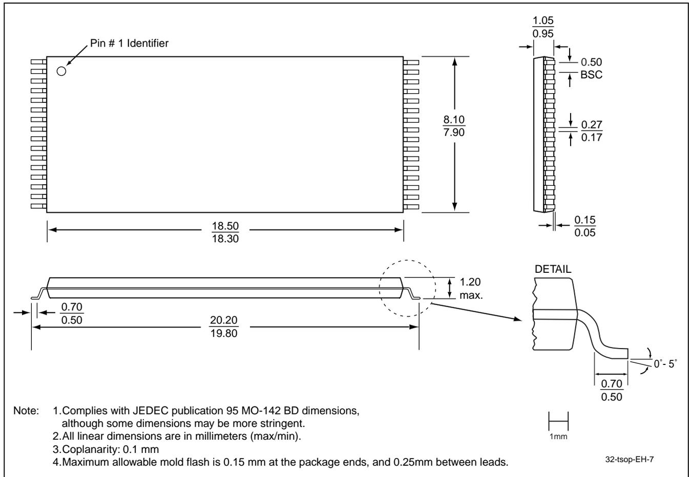
**FIGURE 23: 32-lead Thin Small Outline Package (TSOP) 8mm x 20mm**
