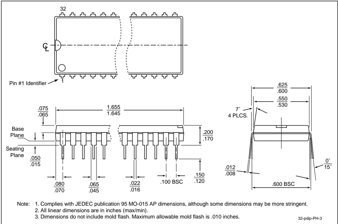
**FIGURE 24: 32-pin Plastic Dual In-line Pins (PDIP)**
