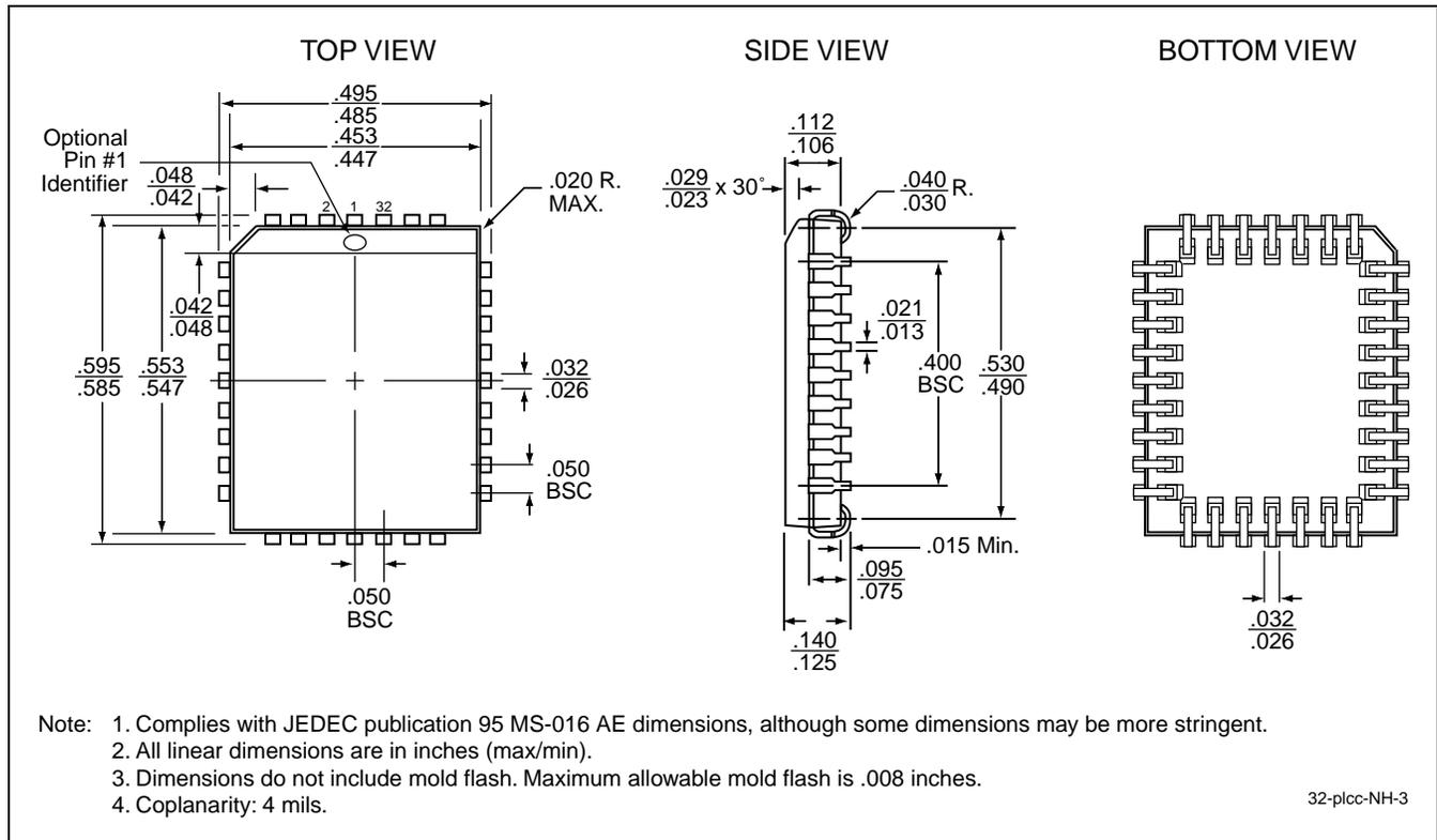
**FIGURE 21: 32-lead Plastic Lead Chip Carrier (PLCC)**
