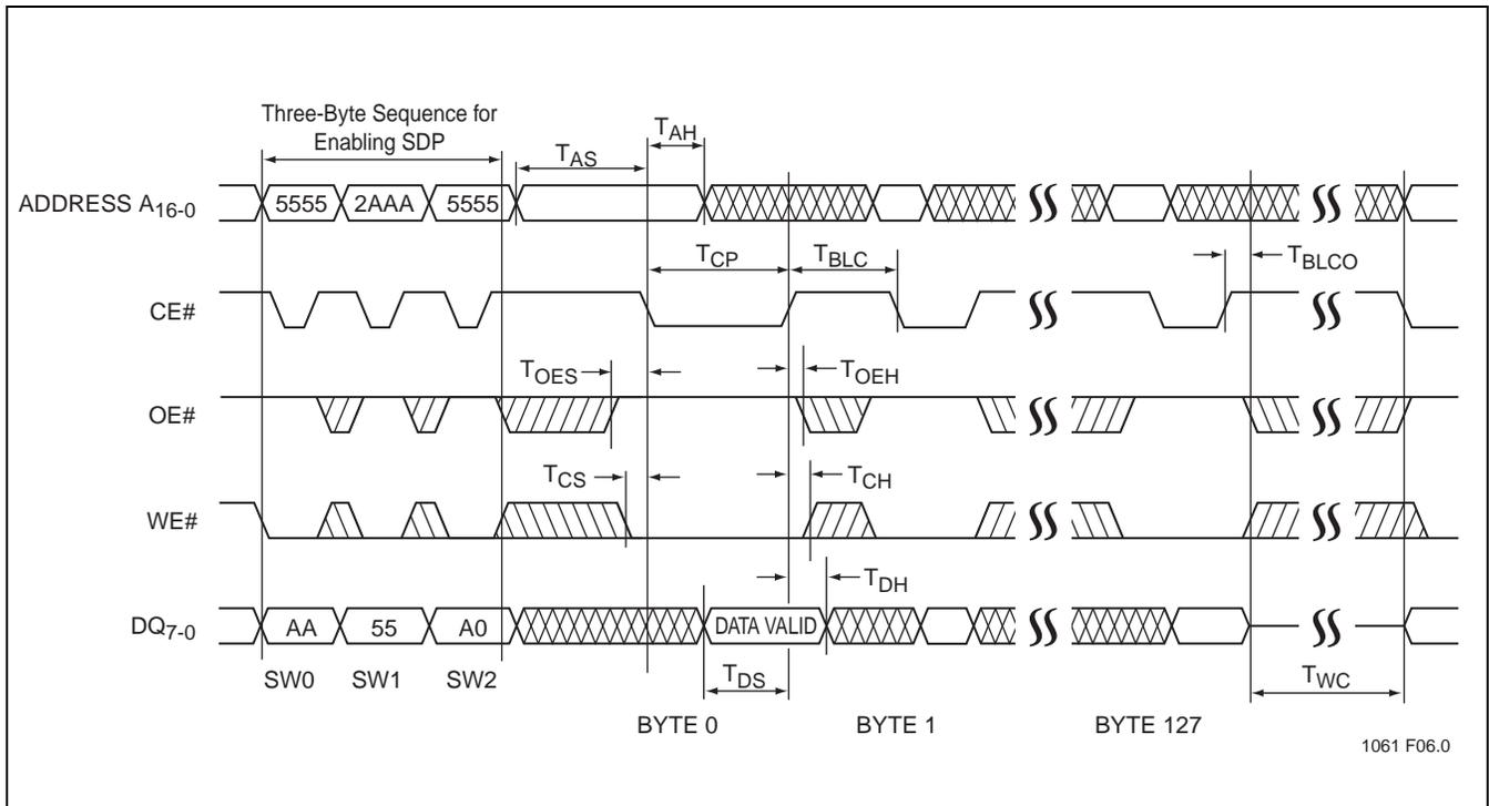
**FIGURE 7: CE# Controlled Page-Write Cycle Timing Diagram**
