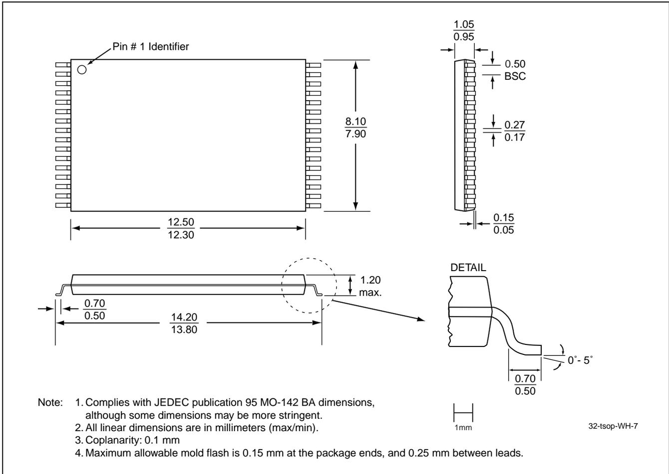
**FIGURE 22: 32-lead Thin Small Outline Package (TSOP) 8mm x 14mm**
