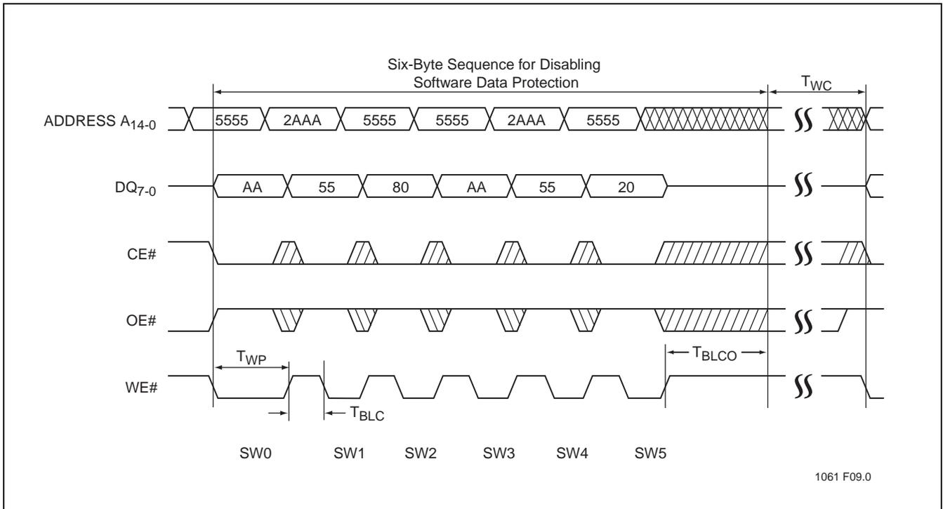
**FIGURE 10: Software Data Protect Disable Timing Diagram**
