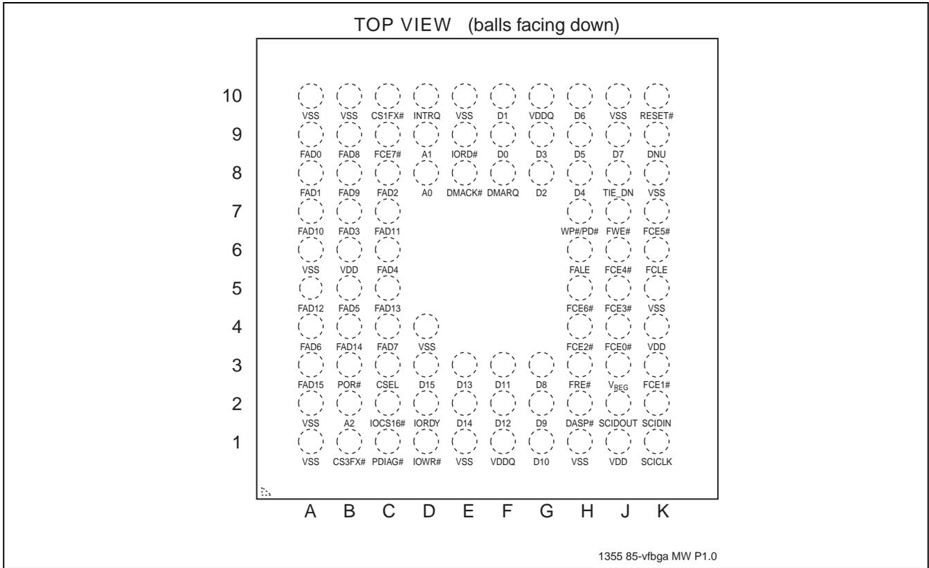
**FIGURE 3: PIN ASSIGNMENTS FOR 85-BALL VFBGA (MW)**
