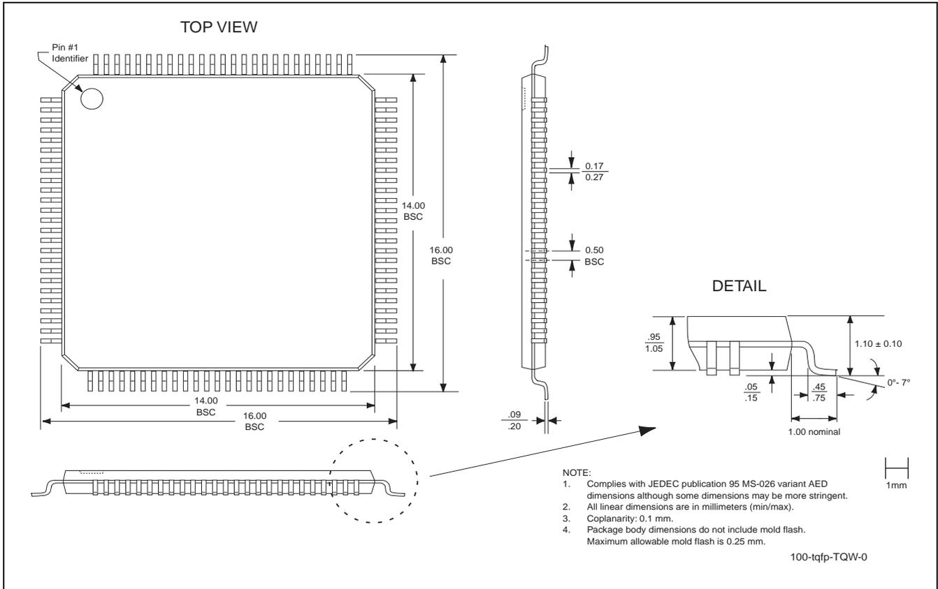
**FIGURE 10: 100-lead Thin Quad Flat Pack (TQFP)**
