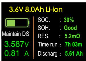
Generally, a complete maintenance process takes about 30 hours. After the process is completed, the battery capacity Ah value is the most accurate. Press <Up> key, the display screen will display the recorded complete battery charging/discharging curves.
