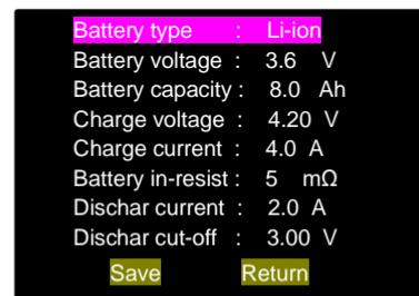
**[Battery type]:** Select of one from LiFePO4, Li-Ion, Pb-Acid, NIMH, NICD,
