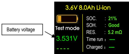
The fast tested SOC percentage is built based on the measured battery voltage and equipment learning. This SOC is calculated by looking up the voltage-SOC table.
