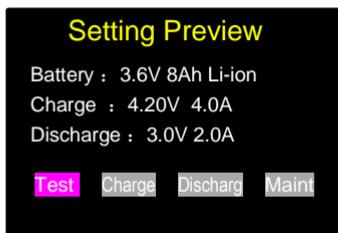
If the parameters are correct, users can select the four listed in the menu according to their task requirement functions. Use <Up>, <Down> and <Enter> to select and run. If errors are found in the preview parameters, please press <Enter> for more than 2 seconds, and the system will return to the home page to reset battery parameters.
