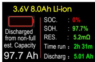
When discharge battery from non-full state, after discharged empty, it will get an estimated capacity.
