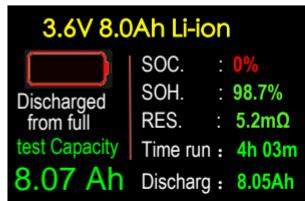
When discharge battery from full charged state, after discharged empty, it will get an accurate capacity.
