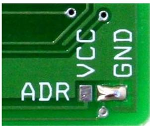
However, if you wish to connect more than two modules on the bus, the external address can be use to connect up to four modules. That is total of 16-digit. To use external address selection, remove all of the solder bridge from ADR pads. Connect voltage to the ADR pin 5 according to the table below.
