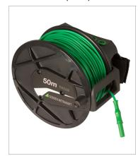
50 m measurement cable coiled onto a plastic drum. Connection to the inside end of the cable is made possible with two sockets integrated into the drum. The other end is equipped with a banana plug.
