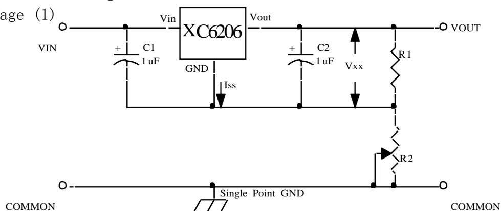
$$V_{out} = V_{xx}(1 + R_2/R_1) + I_{SS}R_2$$
