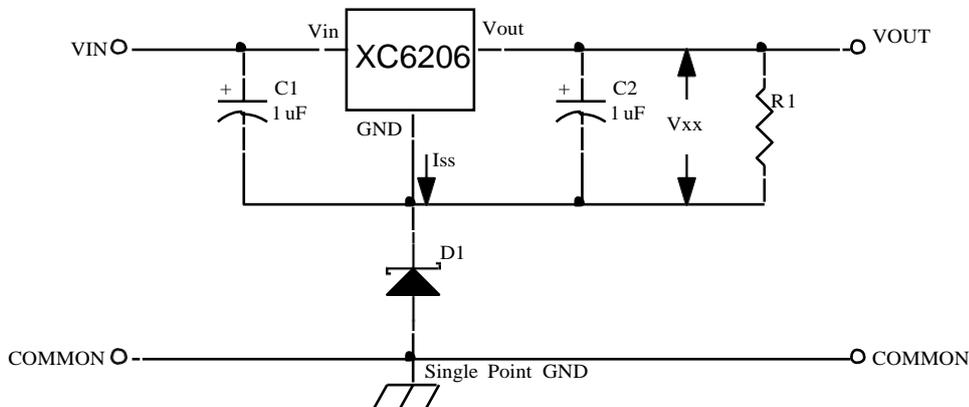
$$V_{out} = V_{xx} + V_{D1}$$
