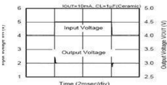
Load transient input response characteristics
