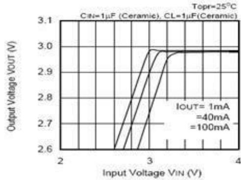
3. Dropout voltage and output current
