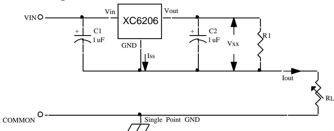
$$I_{out} = V_{xx} / R_A + I_{ss}$$
