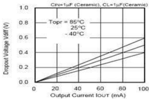
4. Dropout voltage and output voltage
