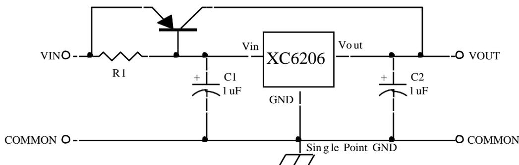
3. Circuit for increasing output voltage (1)
