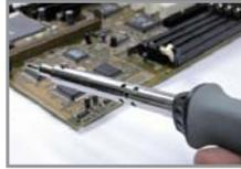
Dual heat soldering iron
