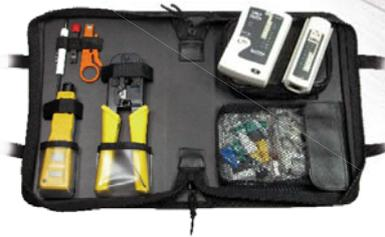
Multi-Network Cable Tester for RJ45, RJ11 (UTP / STP). Adjustable Impact Punch Down Tool, with 110 / 66 blade. 3 Way 7.5" Crimping Tool for 8P / 6P / 4P. Stripper for Wire dia. 5-6.2mm top end 110 / 88 Insertion. 2 in 1 mini Screwdriver Slotted and Phillips. 50 Piece RJ45 (8P8C) Modular Plugs. 20 Piece Color Strain Relief. Components Pocket. Zipper Vinyl Case.
