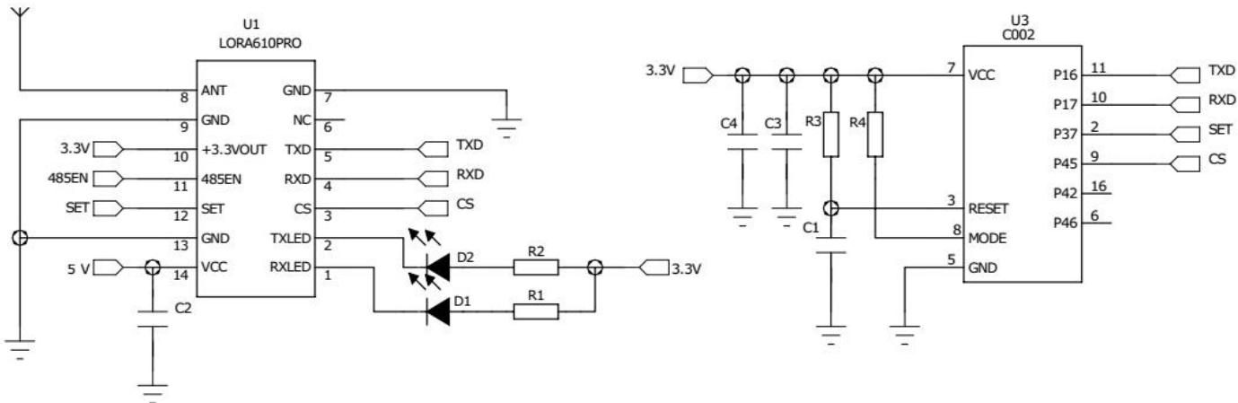
Note: The ground wire of the module must be connected to the digital ground of the device.
