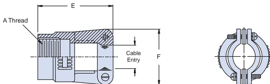
**TABLE I: Shell Size, Cable Entry and Backshell Dimensions**
