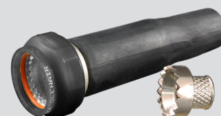
317V111 Piggyback Boot Adapter These composite, self-locking backshells have a drop-in banding adapter and are supplied with pre-attached shrink boot Page 137
