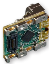
PCB-mount opto-electronics feature Samtec high-speed surface-mount connectors
