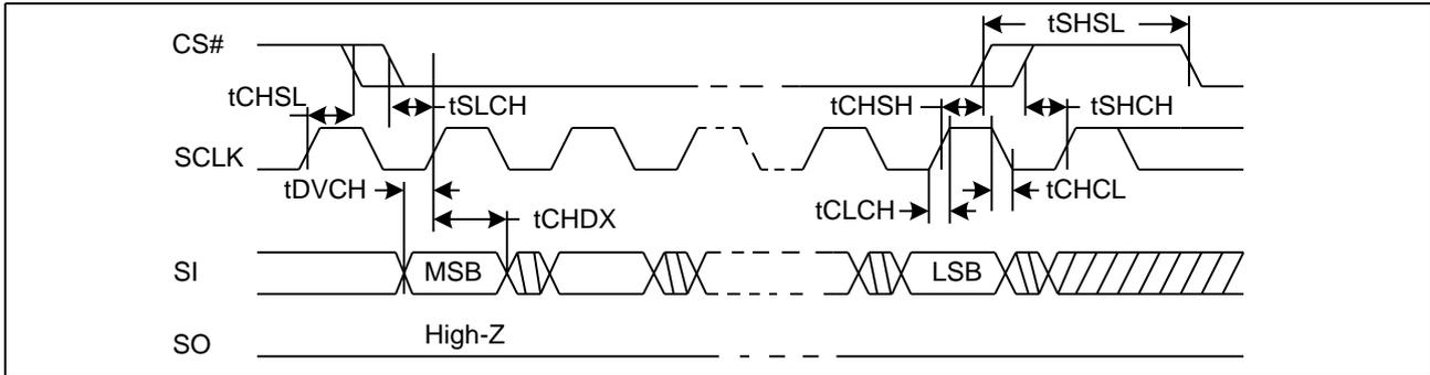
Figure 44. Output Timing
