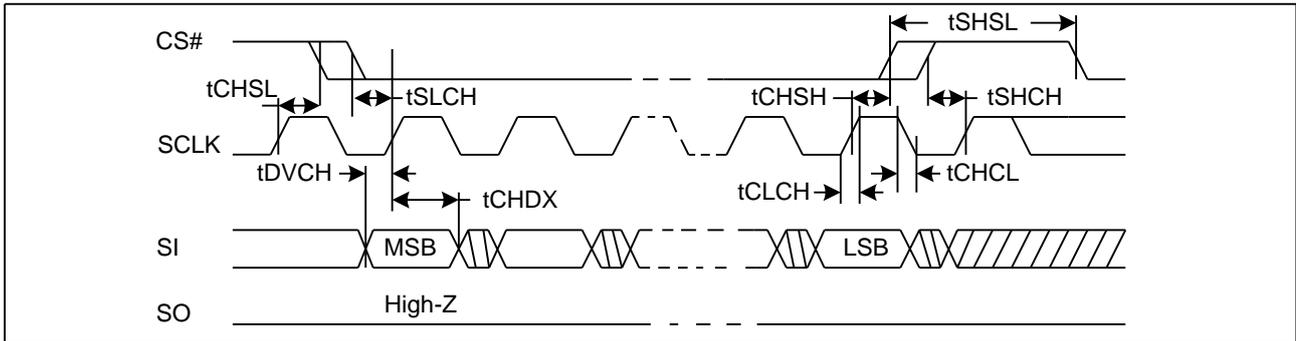
**Figure 40. Output Timing**
