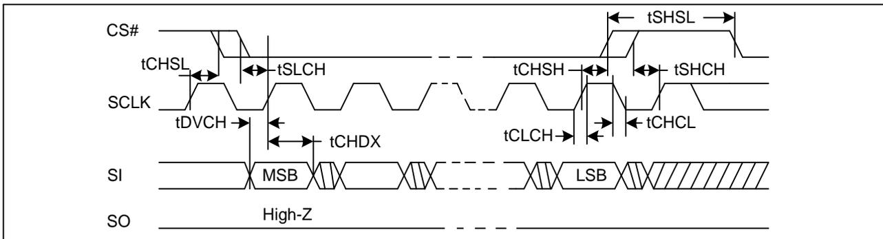
**Figure 39. Output Timing**
