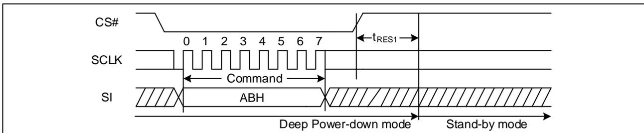
**Figure 24. Release Power-Down/Read Device ID Sequence Diagram**
