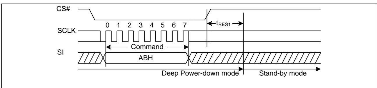
Figure26. Release Power-Down/Read Device ID Sequence Diagram
