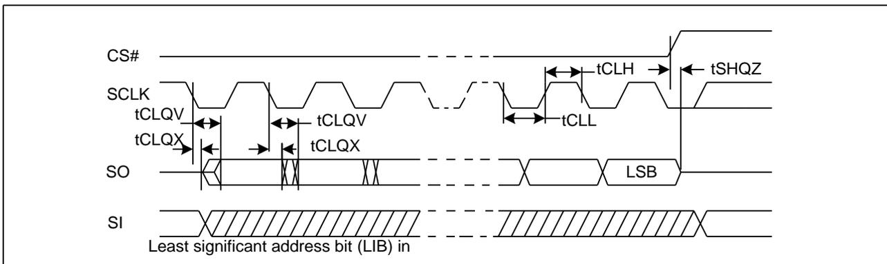
**Figure 43. Resume to Suspend Timing Diagram**
