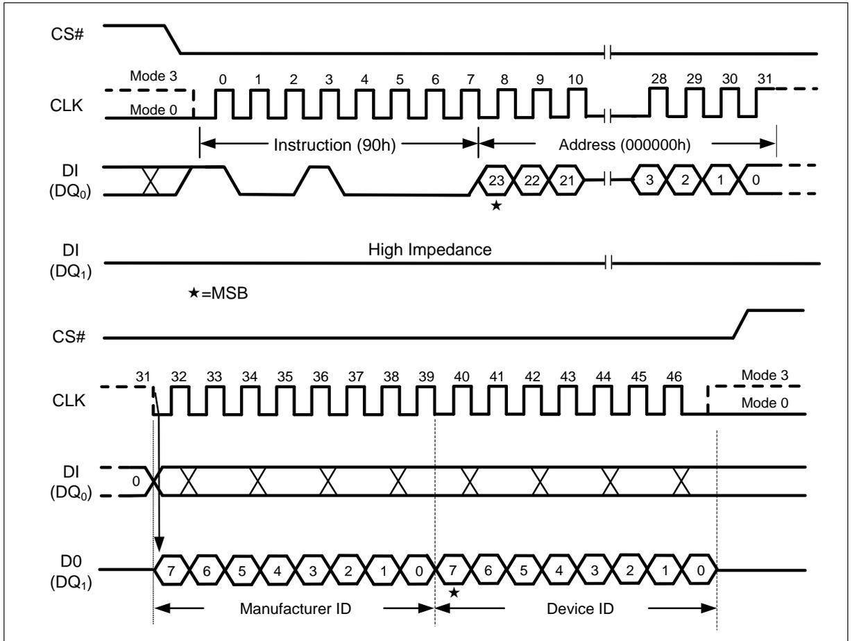
Figure 45 Read Manufacturer / Device ID Instruction (SPI Mode)
