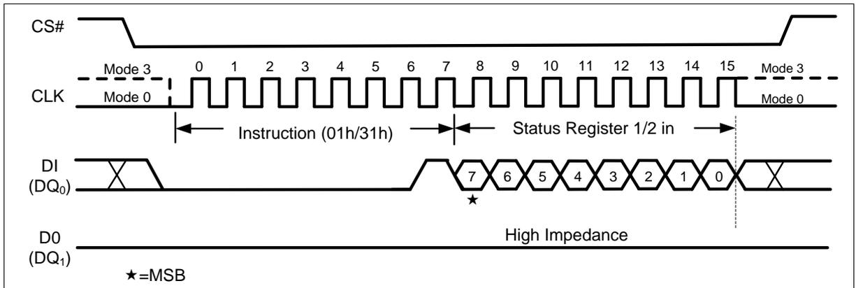
Figure 12 Write Status Register Instruction (SPI Mode)
