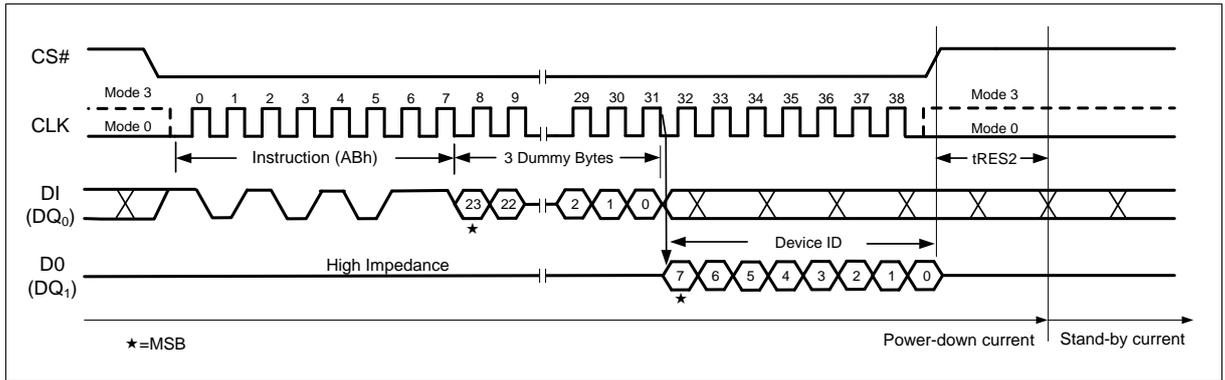
Figure 43 Release Power-down / Device ID Instruction (SPI Mode)
