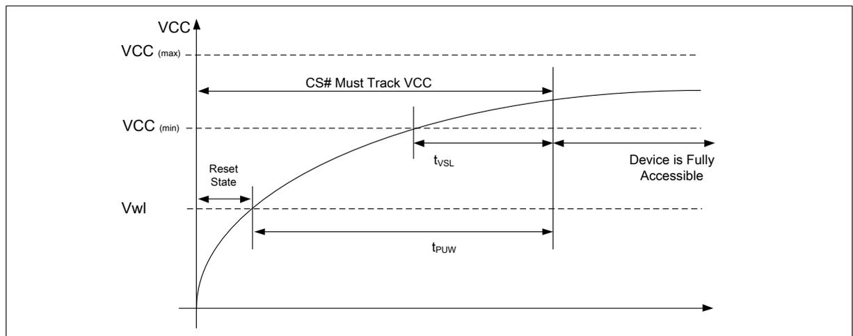
Figure 62 Power-up Timing& Power Up/Down and Voltage Drop
