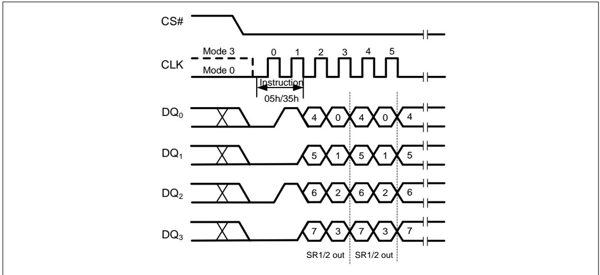
Figure 11 Read Status Register Instruction (QPI Mode)
