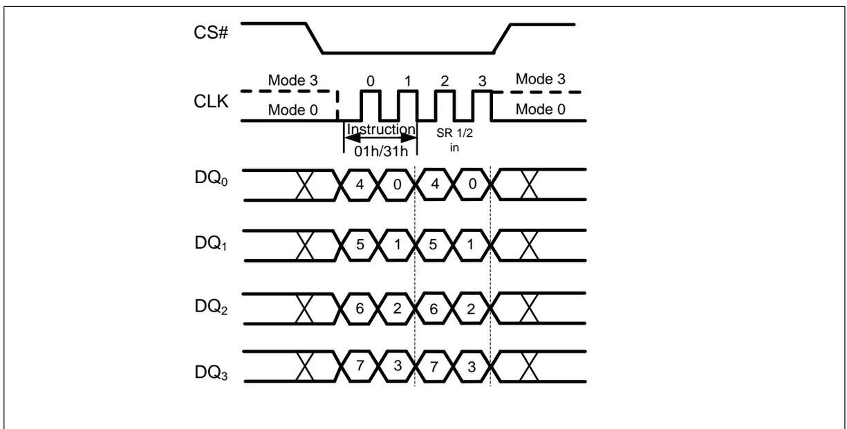
Figure 13 Write Status Register Instruction (QPI Mode)
