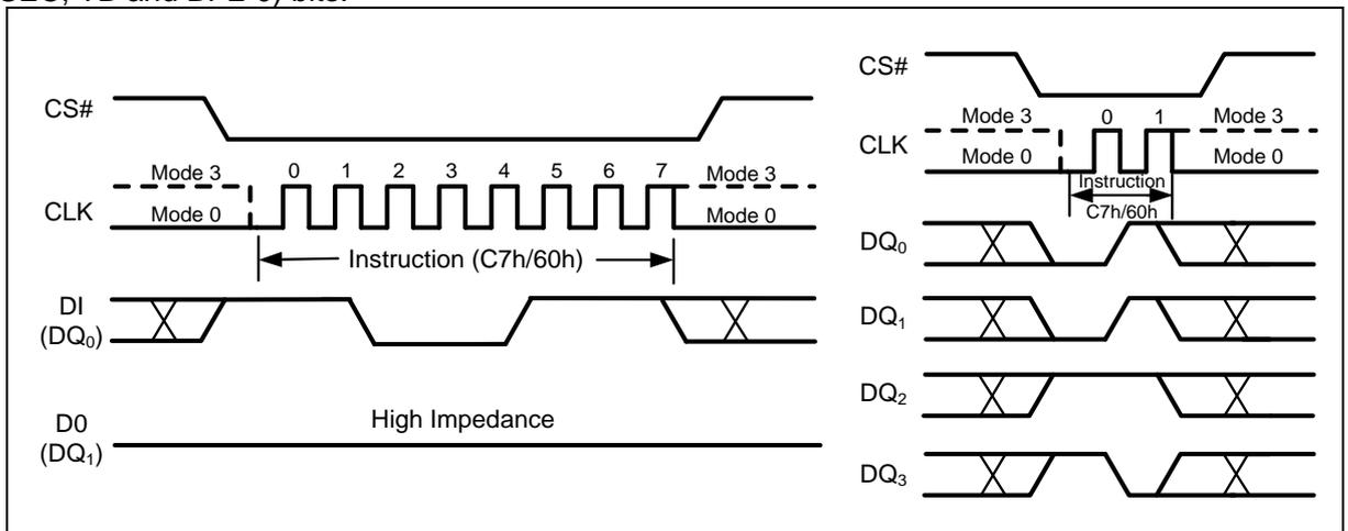
Figure 38 Chip Erase Instruction for SPI Mode (left) or QPI Mode (right)
