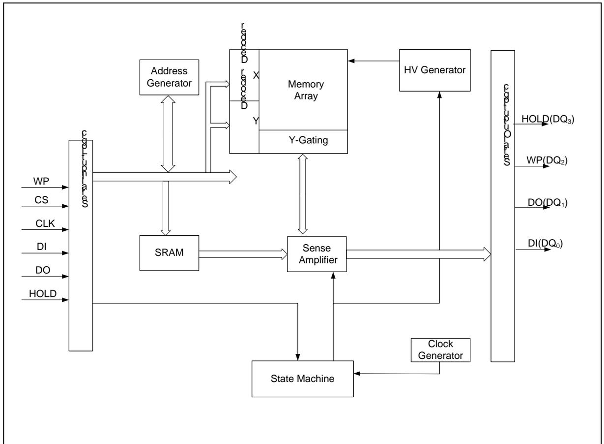
Figure 1 FM25Q04B Serial Flash Memory Block Diagram
