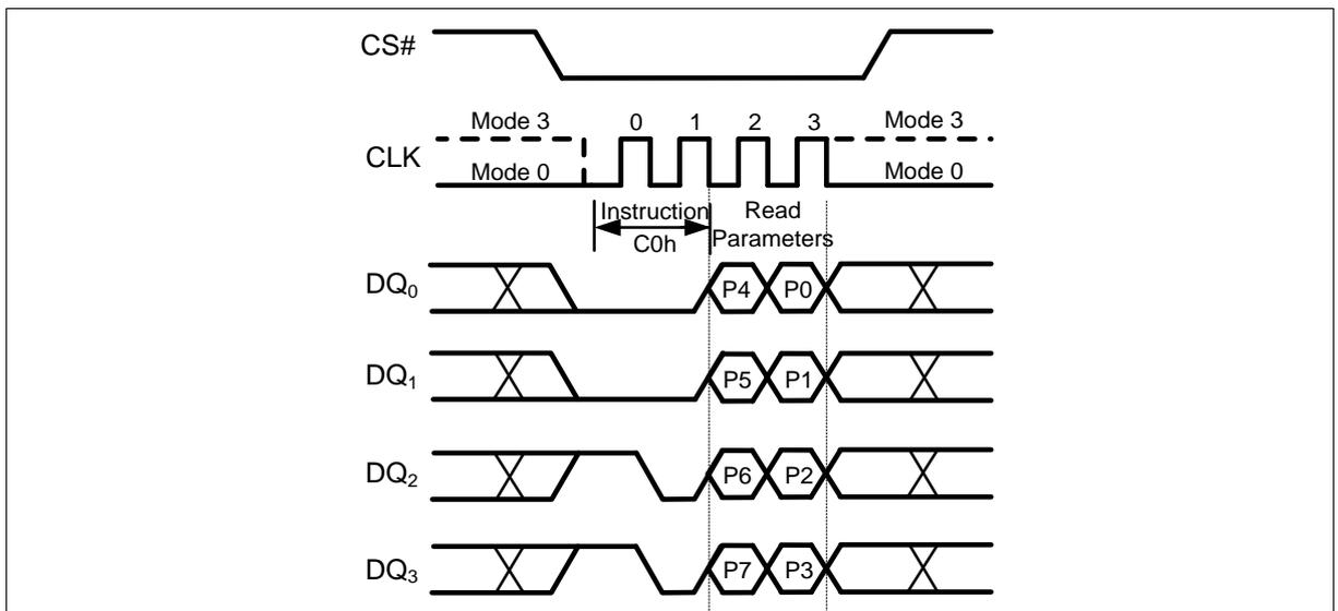
Figure 56 Set Read Parameters Instruction (QPI Mode only)
