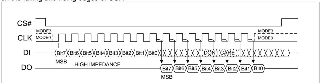
Figure 3 The difference between Mode 0 and Mode 3
