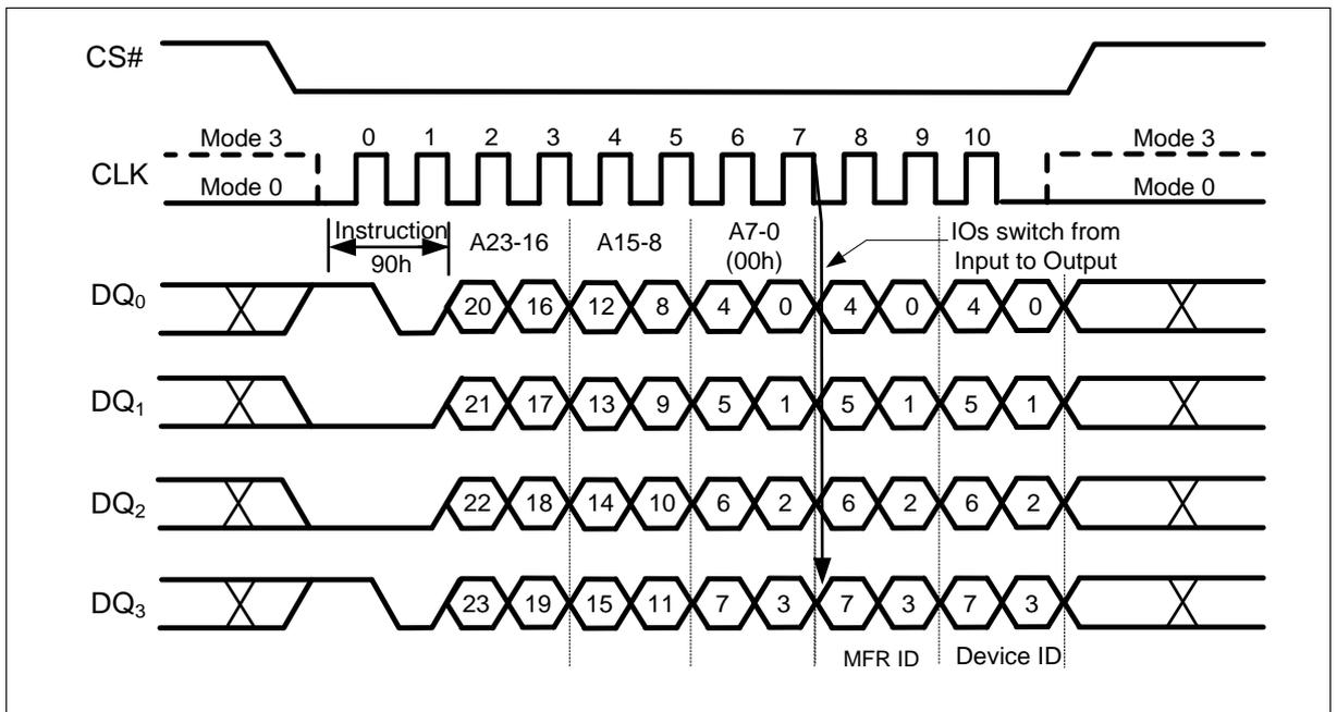
Figure 46 Read Manufacturer / Device ID Instruction (QPI Mode)
