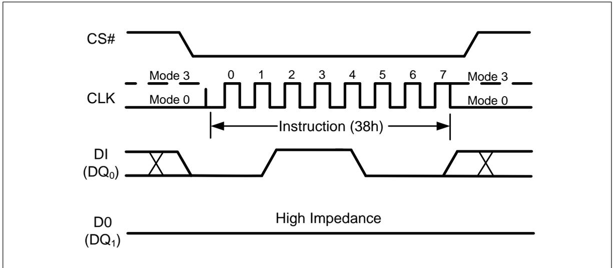
Figure 58 Enable QPI Instruction (SPI Mode only)
