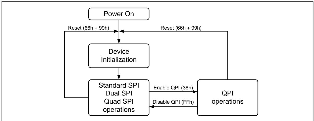
Figure 2 FM25Q04B Serial Flash Memory Operation Diagram
