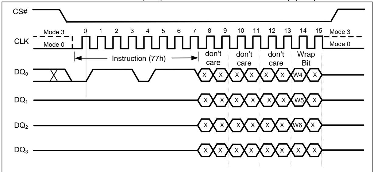
Figure 32 Set Burst with Wrap Instruction (SPI Mode only)
