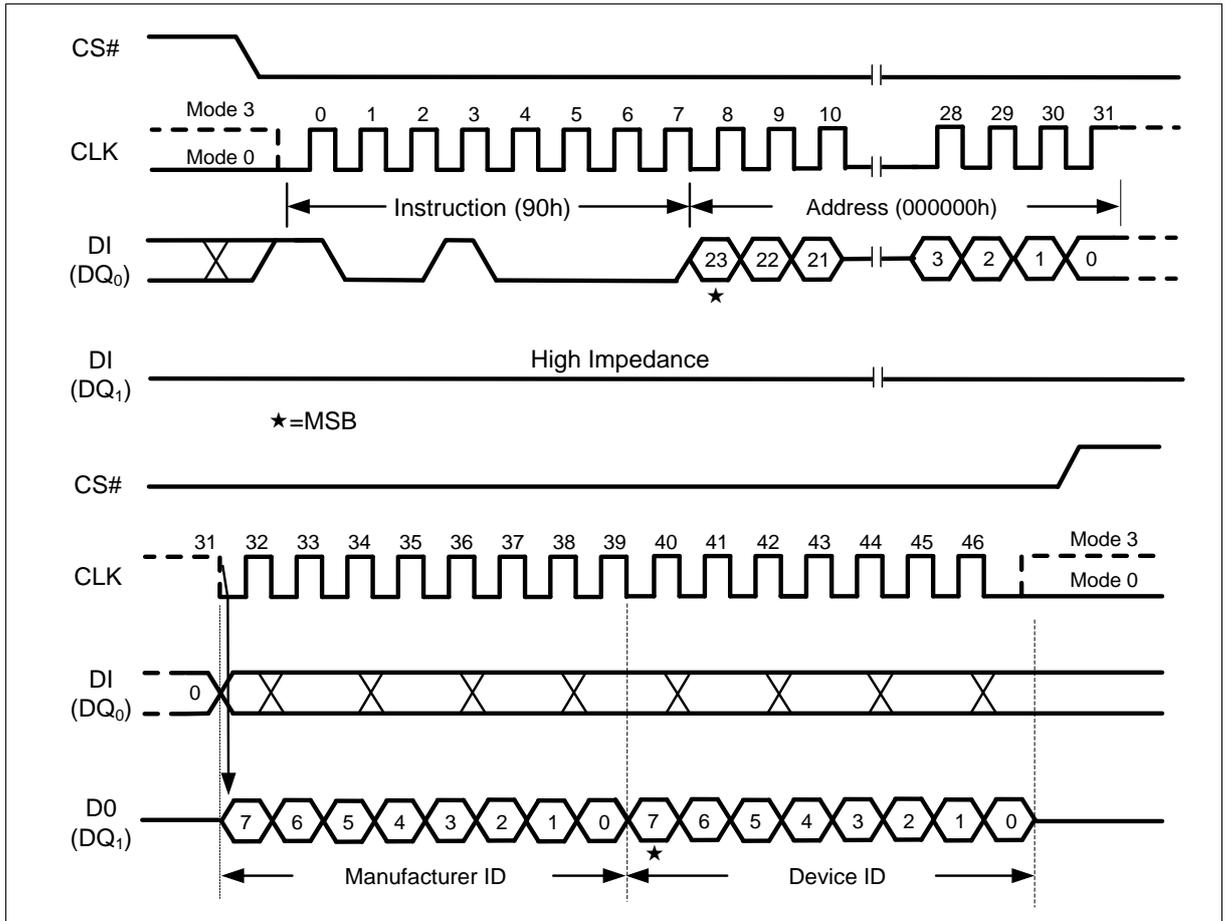
Figure 49 Read Manufacturer / Device ID Instruction (SPI Mode)
