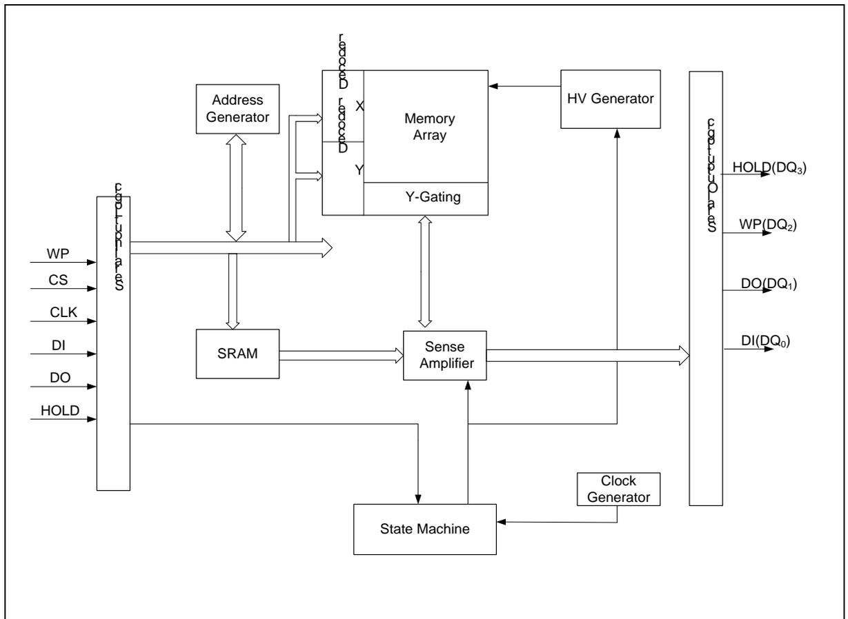
Figure 1 FM25F005A Serial Flash Memory Block Diagram
