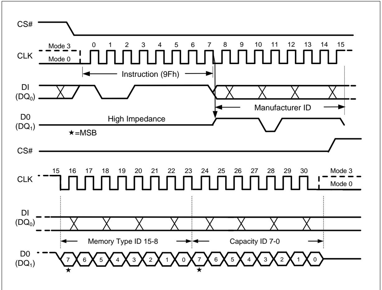
Figure 54 Read JEDEC ID Instruction (SPI Mode)
