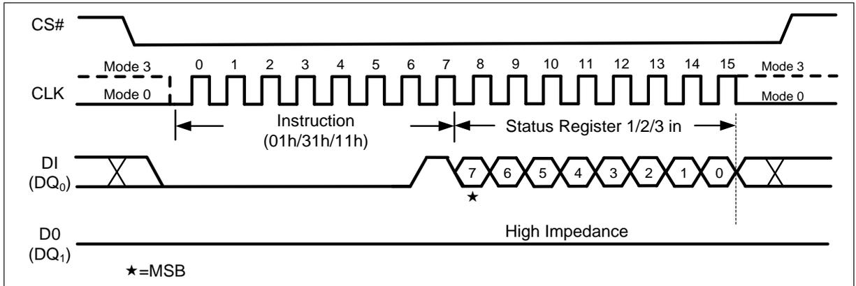
Figure 14 Write Status Register Instruction (SPI Mode)
