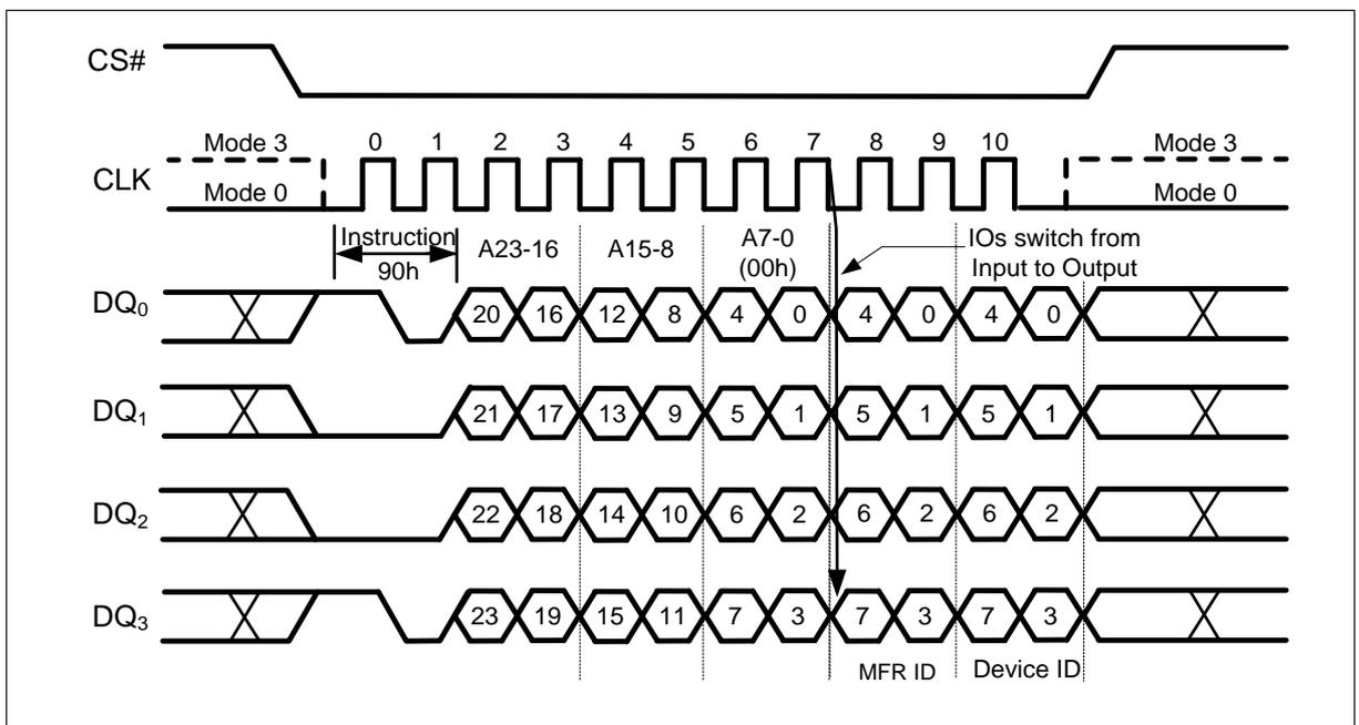
Figure 50 Read Manufacturer / Device ID Instruction (QPI Mode)
