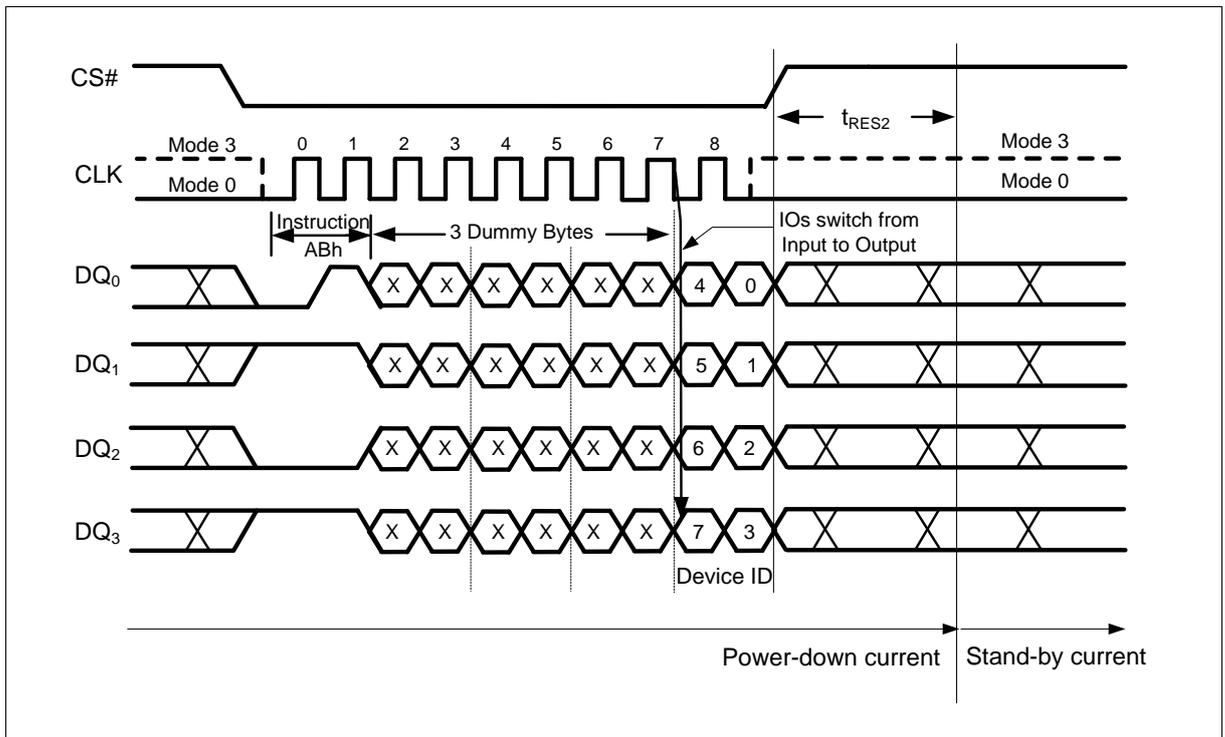
Figure 48 Release Power-down / Device ID Instruction (QPI Mode)
