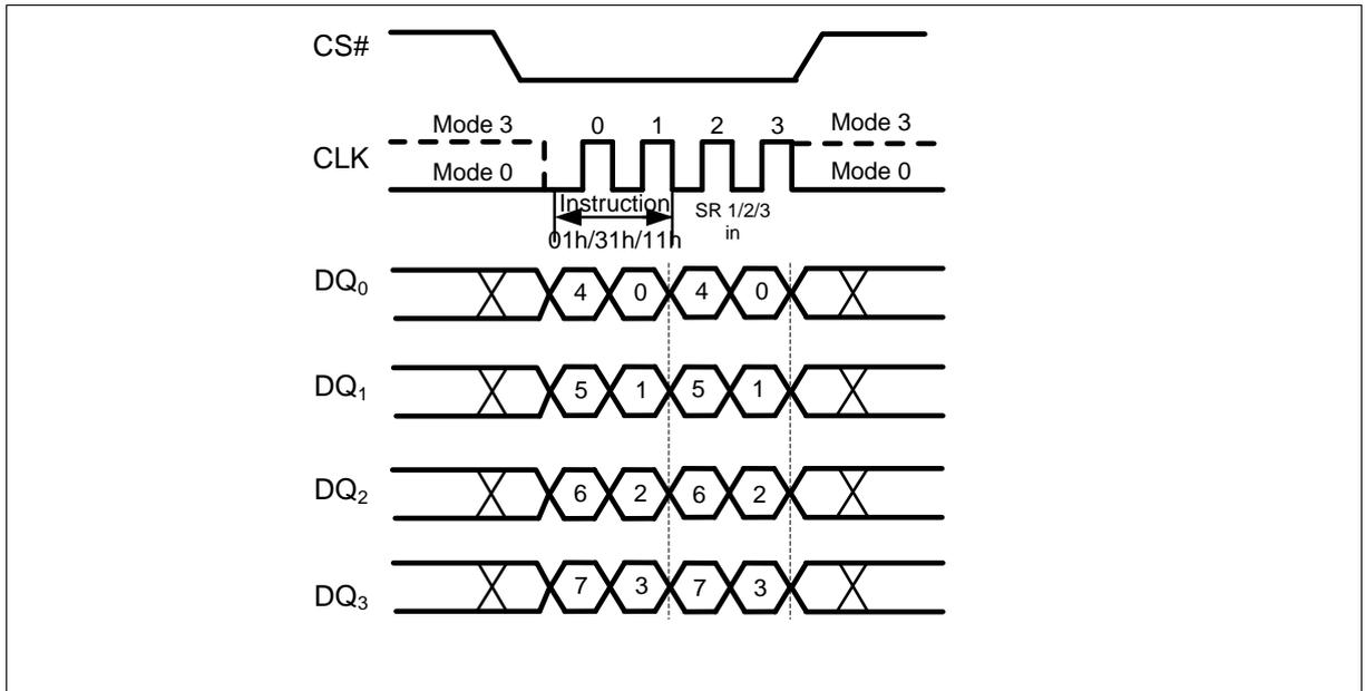
Figure 15 Write Status Register Instruction (QPI Mode)
