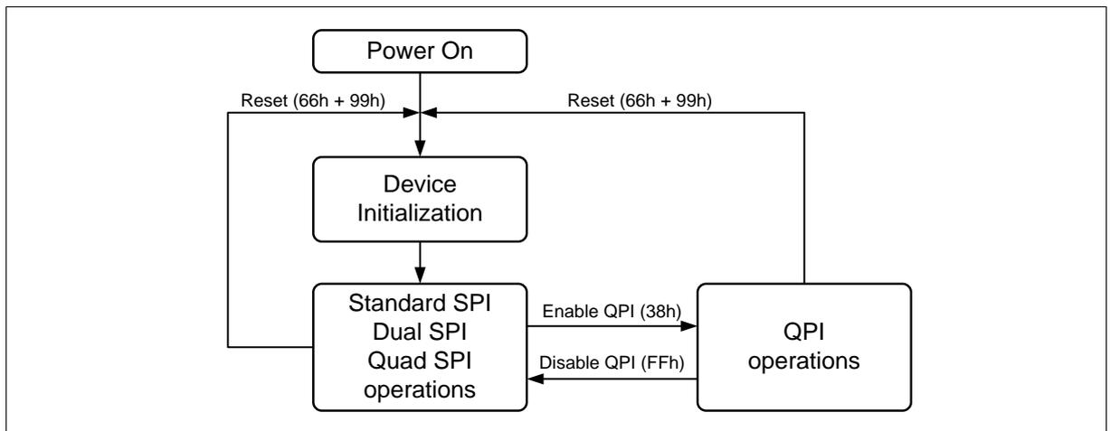
Figure 2 FM25F005A Serial Flash Memory Operation Diagram
