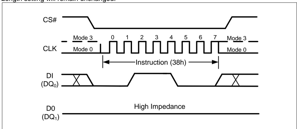
Figure 68 Enable QPI Instruction (SPI Mode only)
