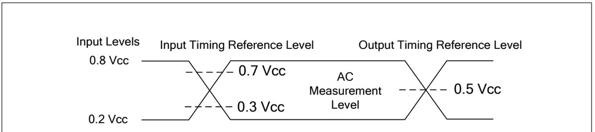
Figure 73 AC Measurement I/O Waveform
