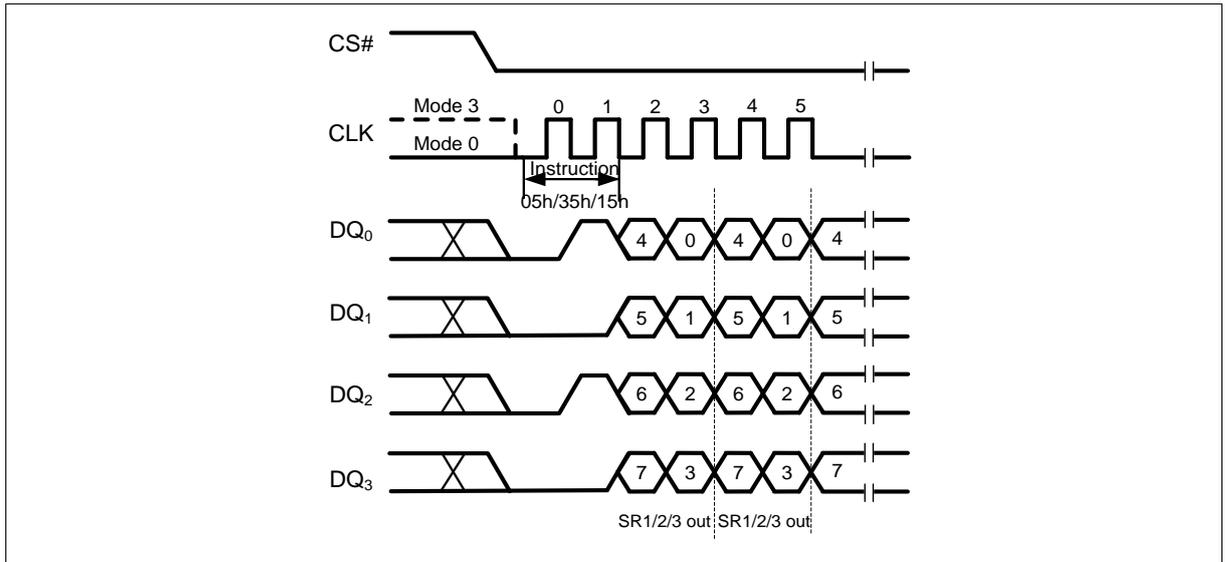
Figure 13 Read Status Register Instruction (QPI Mode)
