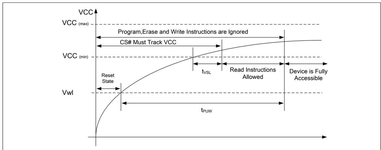
Figure 72 Power-up Timing
