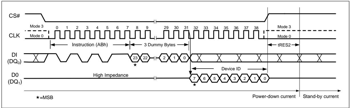
Figure 47 Release Power-down / Device ID Instruction (SPI Mode)
