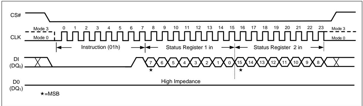
Figure 16 Write Status Register-1/2 Instruction (backward compatible, SPI Mode)
