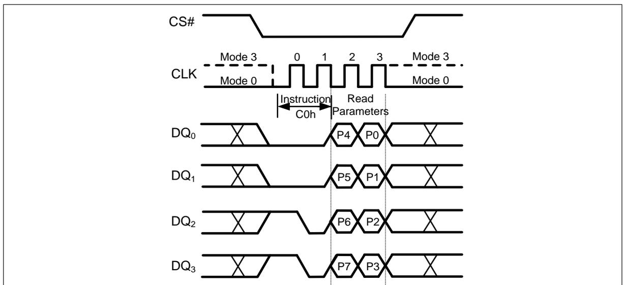
Figure 61 Set Read Parameters Instruction (QPI Mode only)
